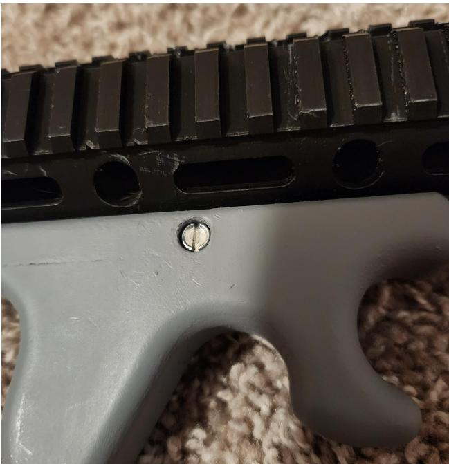
and thread your screw into the nut. Tighten it to point it where it won't move. If you hear plastic cracking, you've tightened it too much.
