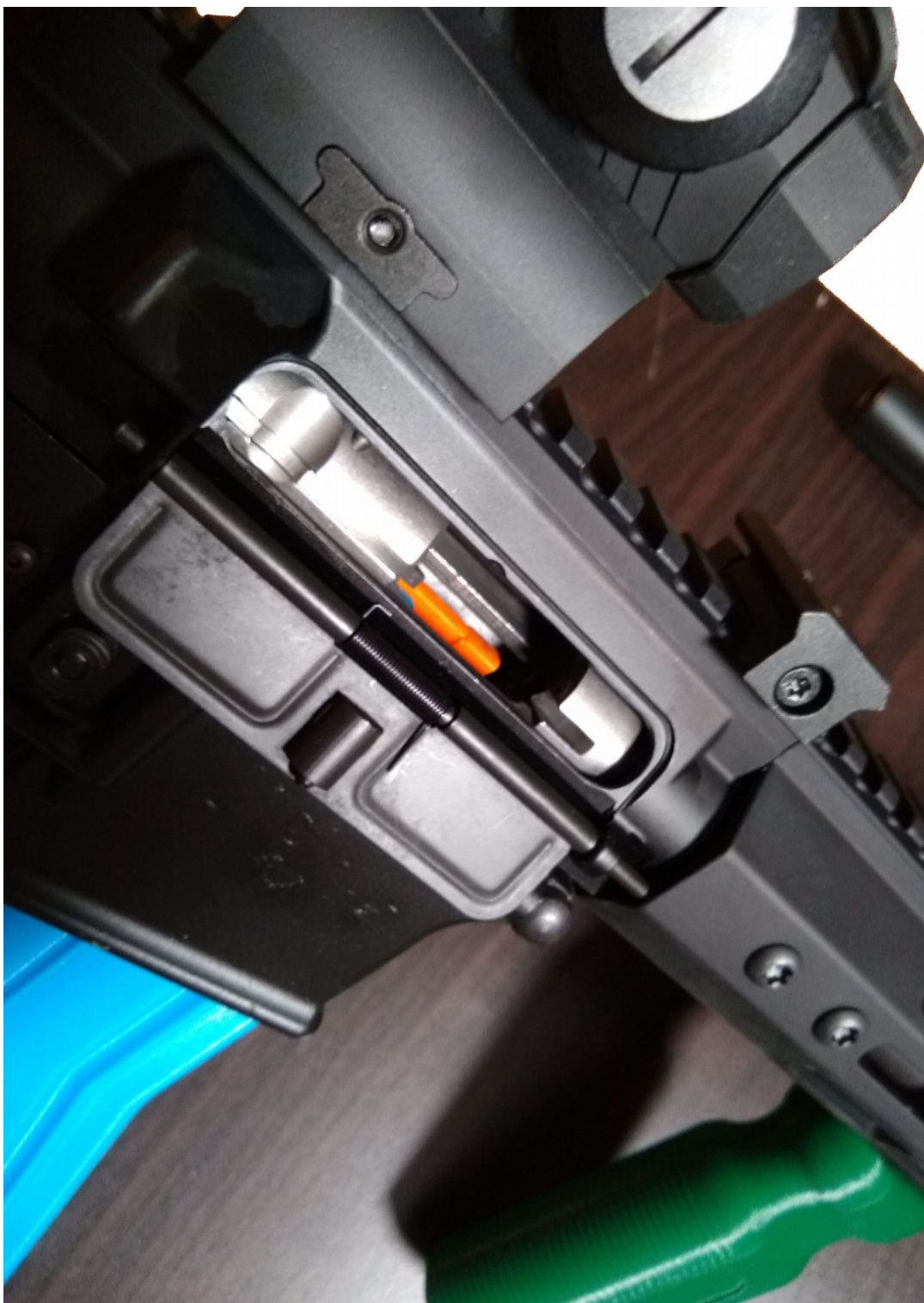
Ex. 2 – Mag (with Follower v2 or v3) locking bolt open
