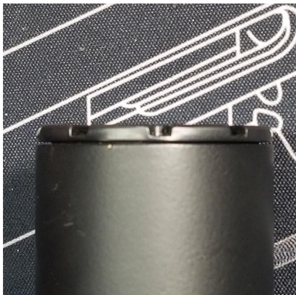
An example of a healthy gap between endcap and tube after hand-tightening.
