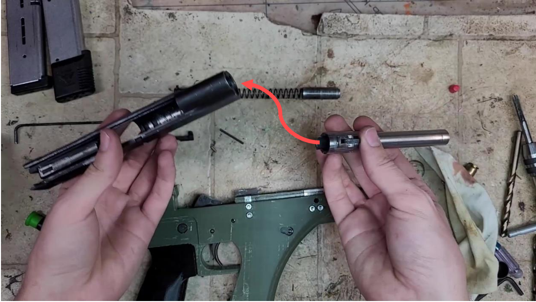
Insert the barrel through the front of the slide. Ensure the barrel link is folded forward.
