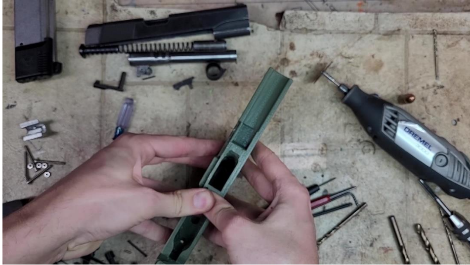
Press the rail down into the frame
