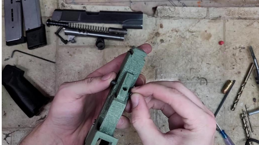
Install the safety selector detent...
