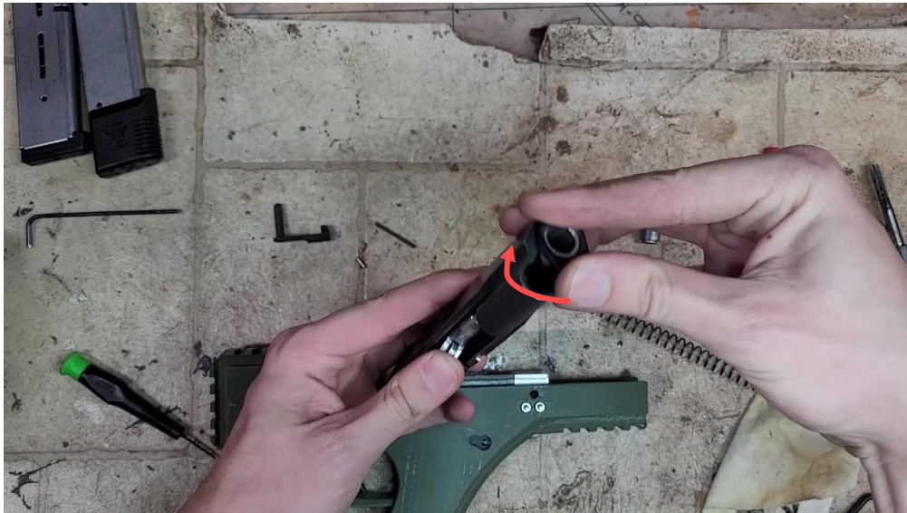
Install barrel bushing and rotate it to the left
