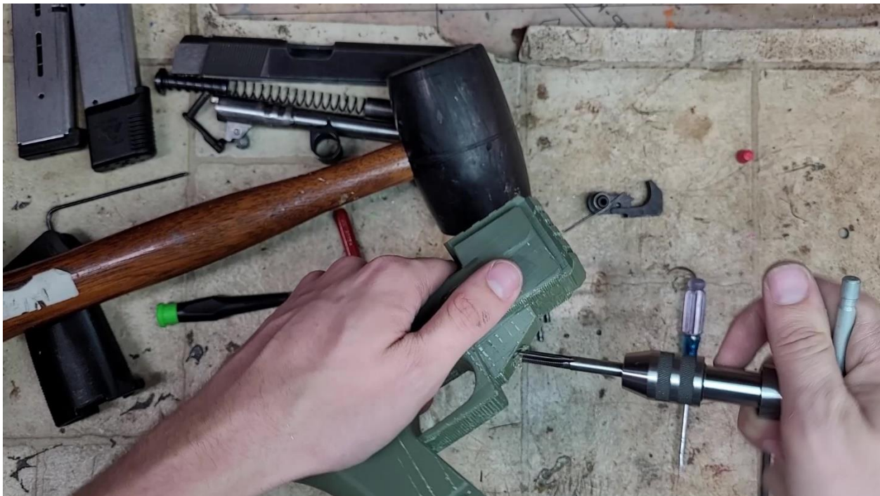
Use a 1/4-28" tap to thread the hole for the pistol grip screw!
