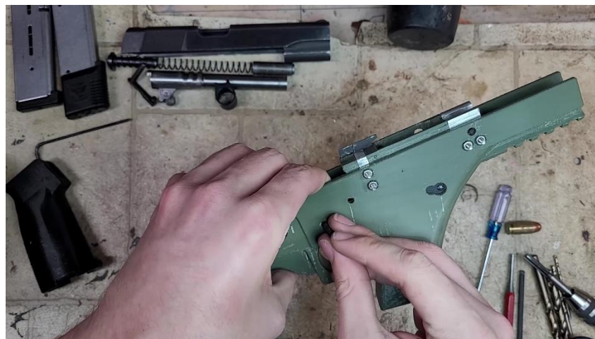
Install the trigger pin so that it retains the trigger and disconnector
