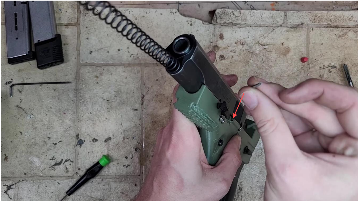
Install the detent spring
