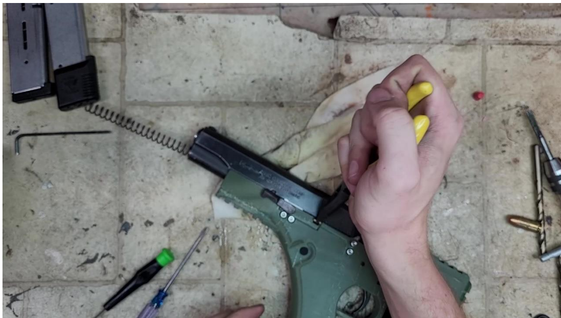
Use pliers to hold the detent in alignment with the hole...
