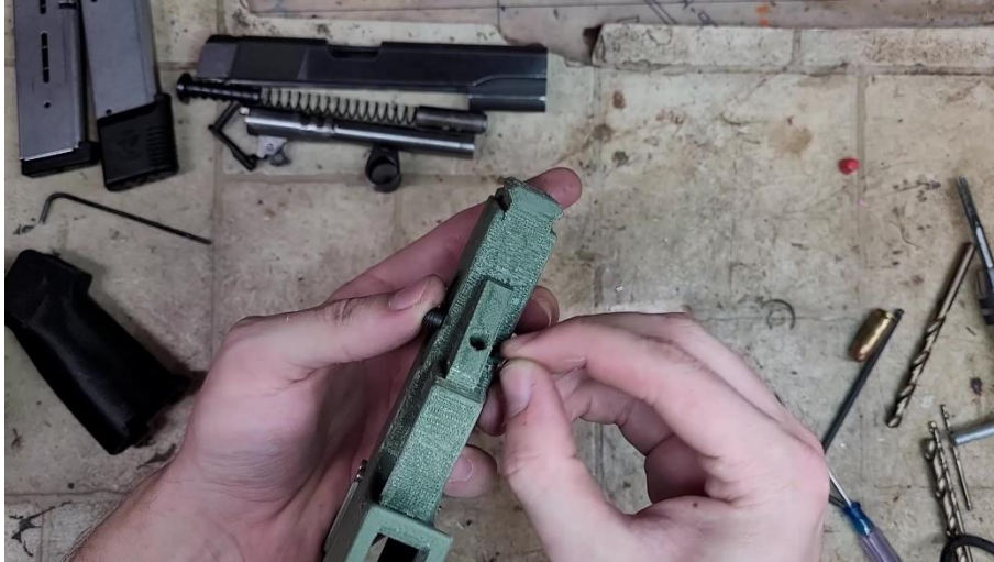
Install the safety selector detent...
