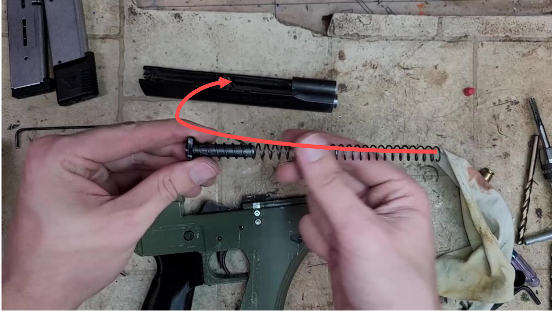
Insert the recoil spring and guide rod
