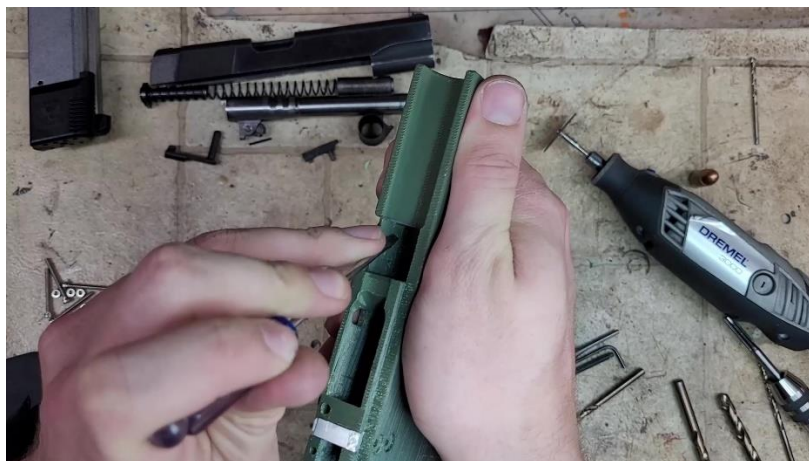
You may need to use a screwdriver to make the corners of the rail pocket square and to ensure all support material is removed from the pocket.
