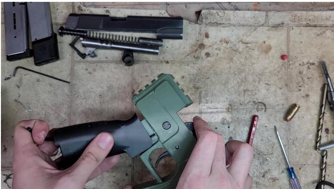
...and then the pistol grip, ensuring that the safety selector detent spring is slotted inside the pistol grip as you install it.
