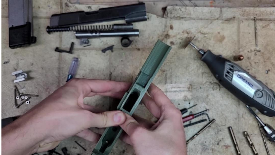
Press the rail down into the frame
