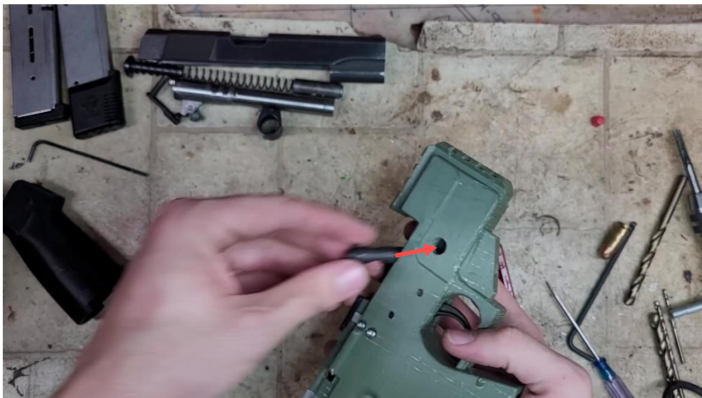
Cock the hammer and insert the safety selector in the safety selector hole
