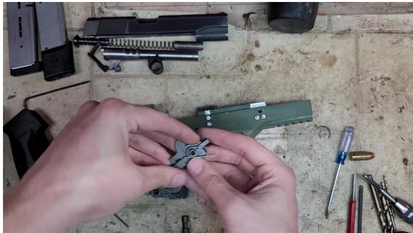
Install AR15 trigger and disconnector, just like on a standard AR15
