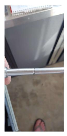
Dry fit barrel pieces together and insert the chamber adapter into the chamber portion of the barrel. Slide your liner down the barrel until it is fully engaged on the chamber adapter. Using a pick/knife/sharpie, mark where the liner will need to be cut. Cut the liner using a small pipe cutter and a drill. Youtube "Cutting a barrel liner" if you need help. Using a chamfering tool, remove the edge from where you cut the liner.
