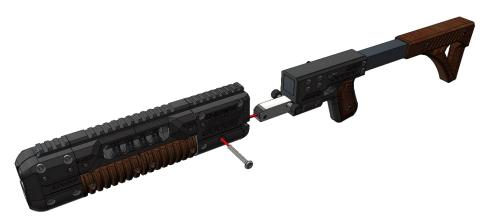
Ensure there is no play in the closed mechanism. Slide the barrel into place and use an empty 410 shell to adjust headspacing. There should be no space between the rear of the cartridge and the breech face. Once the barrel position is adjusted for proper headspacing, use M5 x 40mm bolts to clamp the barrel in place, and use M4 set screws for additional clamping force to ensure it does not shift forward.
