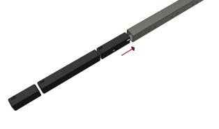
Use 14x M5 x 16mm screws to secure all parts together.
