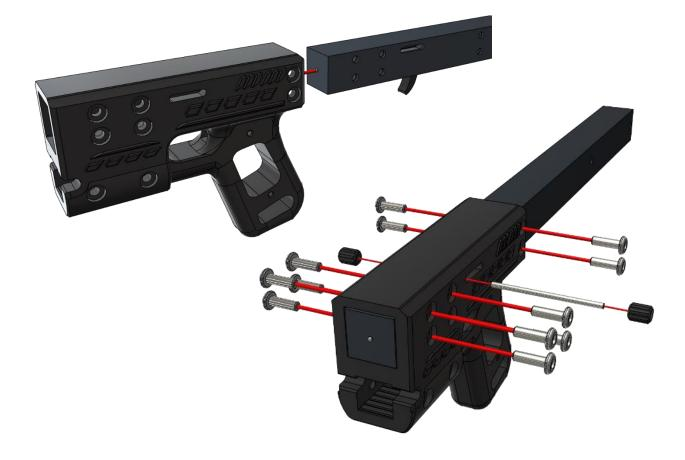
Insert the break barrel latch / hinge assembly into the receiver, and secure with M5 x 16mm screws. If the fit is too loose, you may want to epoxy this section together to eliminate play in the hinge, making sure not to get any epoxy into the sliding latch.
