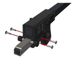
Insert the inner and outer buttstock at the rear, and secure with M5 x 16mm screws. Install the handgrip plug through the rear of the receiver and attach the handgrips with M3 screws.
