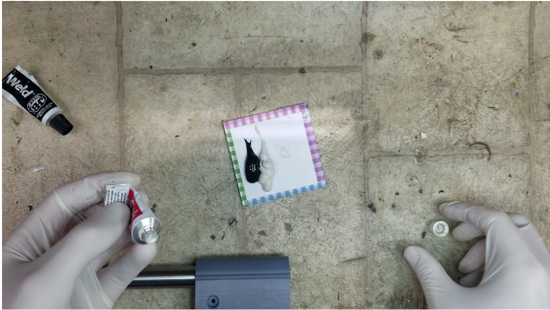
The minimum amount of JBWeld you should use. Mixing more than this amount is a good idea.
