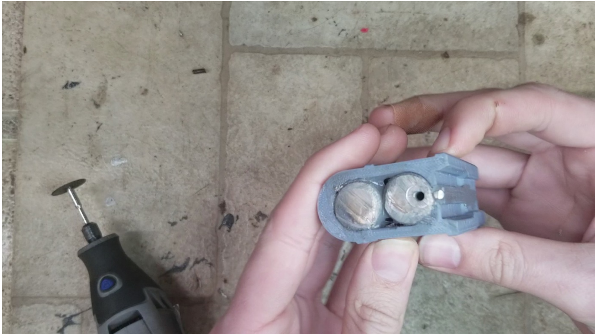
Drill bit filed flat with the bolt face.
