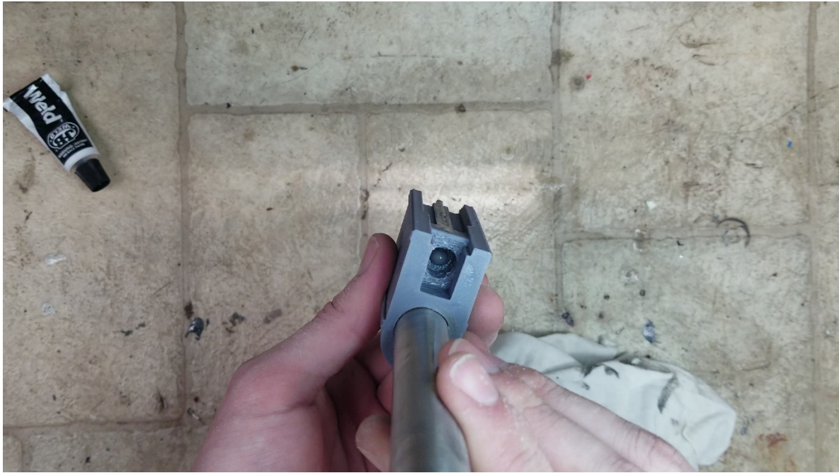
This JBWeld needs to be cleaned out.
