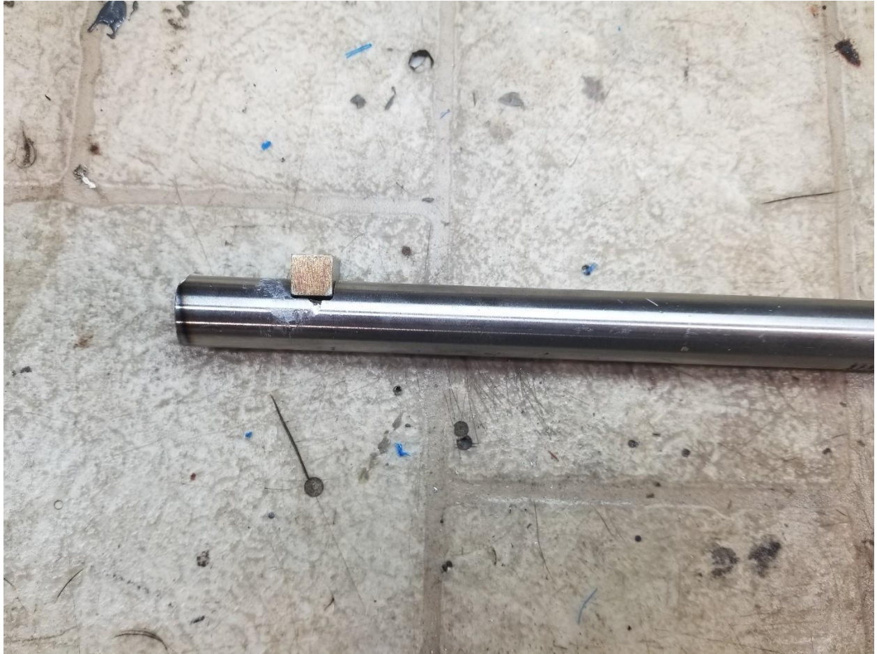
Correct fitment of the bar stock into the slot
