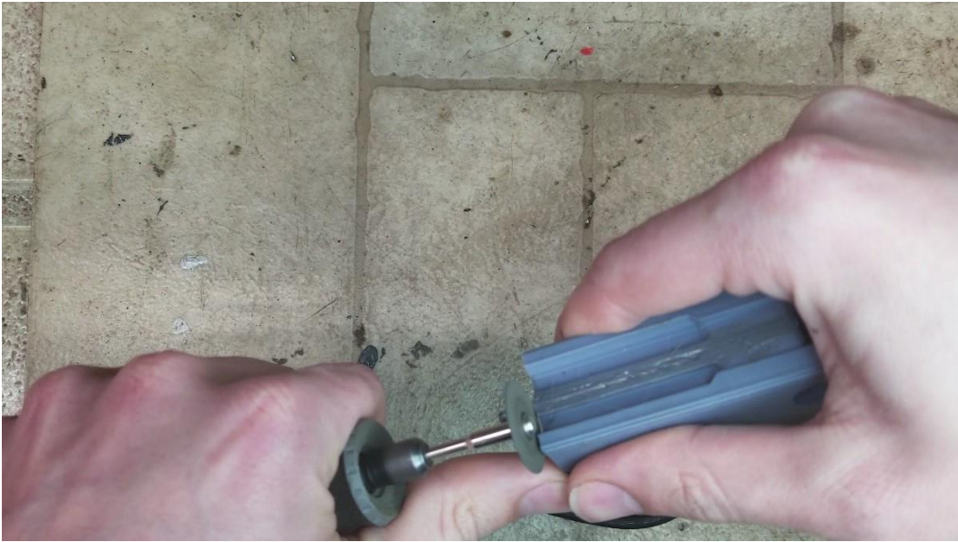
Dremel off most of the drill bit, then use a file to make it flush with the bolt face.
