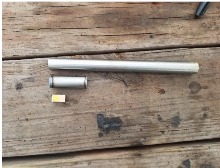
Bolt rods cut to length with bar stock cut to length.
