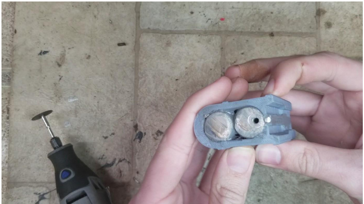
Drill bit filed flat with the bolt face.
