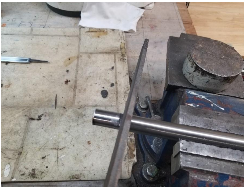
Use a metal file to square up and fine-tune the slot in the bolt rods. File a little, test fit the bar, file some more, etc.
