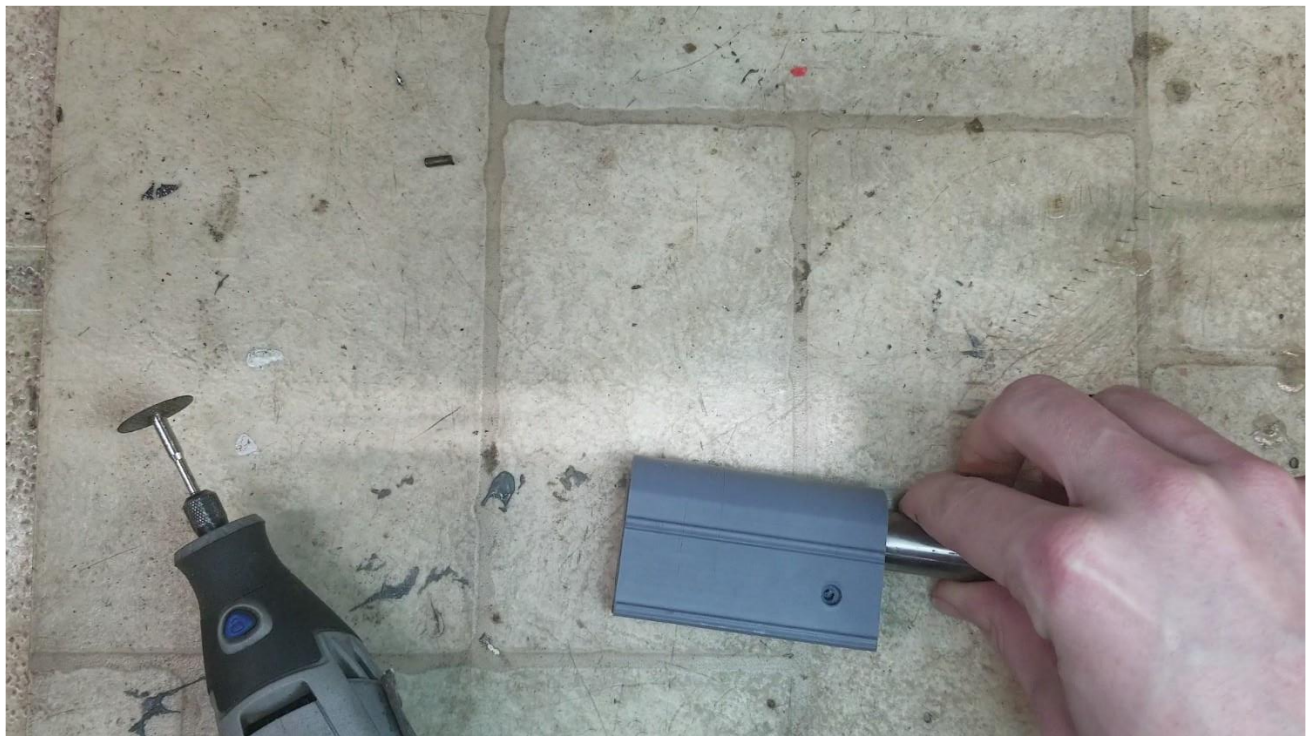
Side view – note that the face of the bolt is flat and the drill bit does not protrude.
