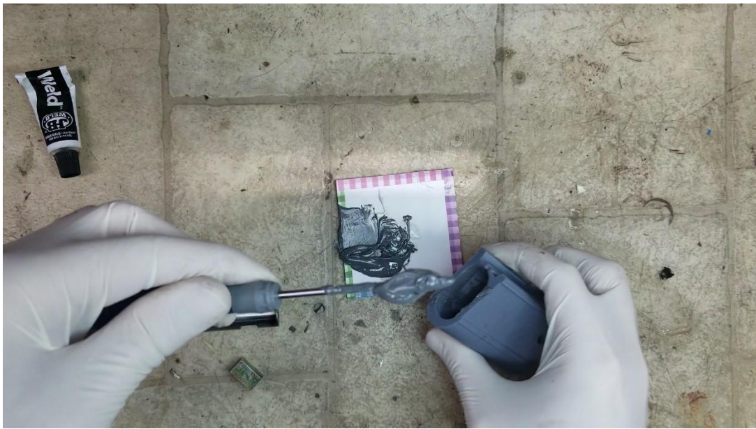
Apply JBWeld to the inside of the housing. Use your tool to spread it out.
