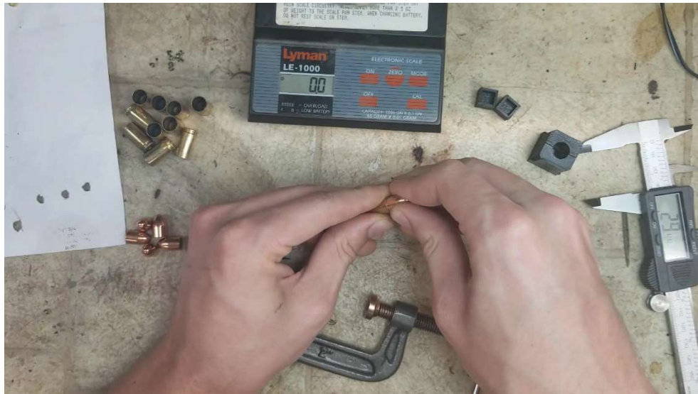
Step 4: Rocking a bullet into the case.
