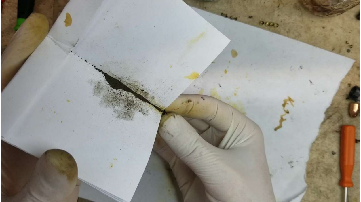
Step 7: Gently tap the priming compound into the primer cup.
