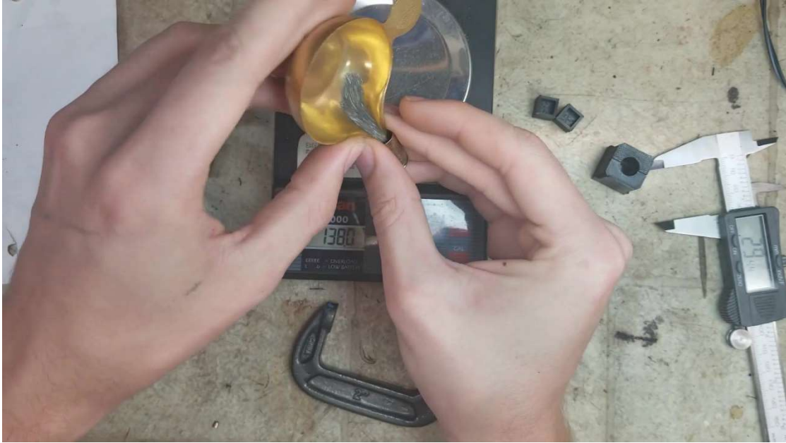
Step 3: Dumping 3.5gr of powder into the case.
