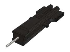
Cut a length of 10mm rod to 8mm length. Cut a channel into the rod to allow the firing pin to pass through (may alternatively be drilled if easier). Secure using CA or Epoxy.
