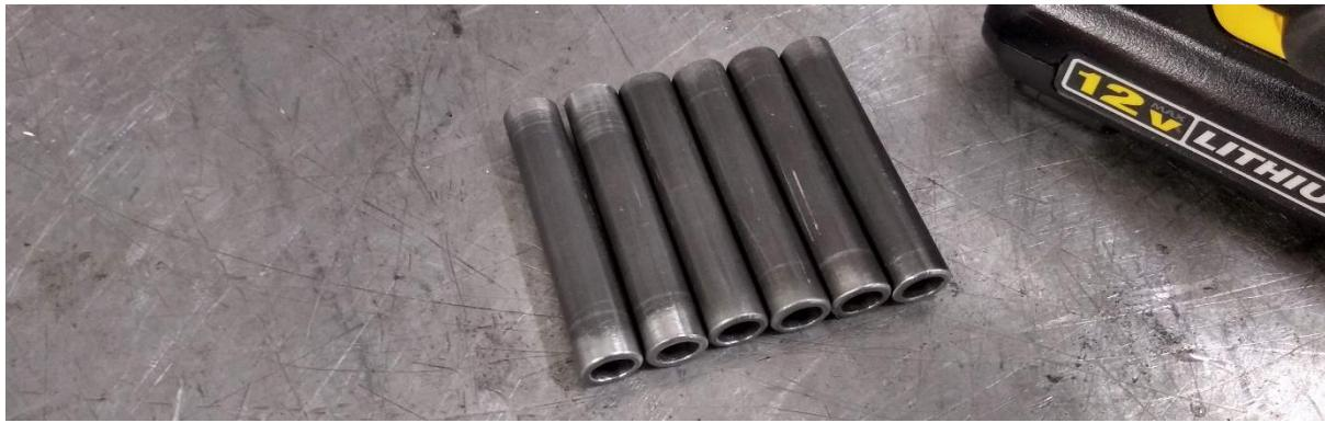
Use a small diameter pipe cutter, rotary tool, or hacksaw to cut the barrel liner into six sections approximately 45mm in length. Use sandpaper or a file to finish each barrel to between 43.5mm-44mm in length. Once each barrel is the correct length, ream a chamber using a #1 wire drill. A vice clamp and BarrelClamp.stl is recommended to hold the barrel while chambering. Chamber depth will be approximately 13mm.
