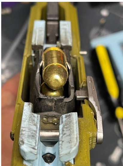
*Slide lock filed down and not touching the magazine (P90 pictured)
