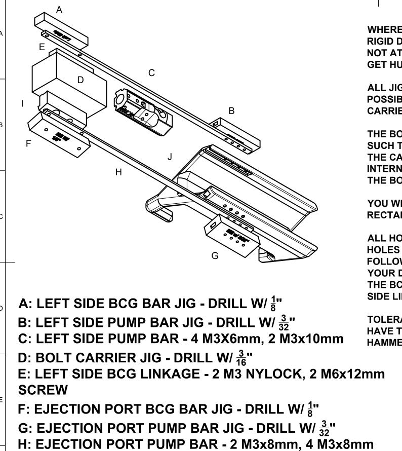
WHERE POSSIBLE, USE A MILL. IF THIS IS NOT POSSIBLE, USE A VERY RIGID DRILL PRESS. A HAND DRILL IS NOT RECOMMENDED. PLEASE DO NOT ATTEMPT TO USE AN ENDMILL IN A HAND DRILL. IF YOU DO AND YOU **GET HURT, IT IS YOUR OWN FAULT.**
