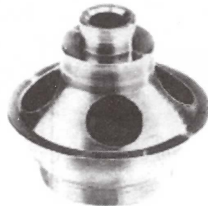
Fig. 24: Circular holes machined in inclined surface by ECM process
