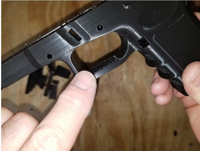
Sand until smooth and trigger clears. Avoid sanding the upper rear portion where trigger safety lever engages.
