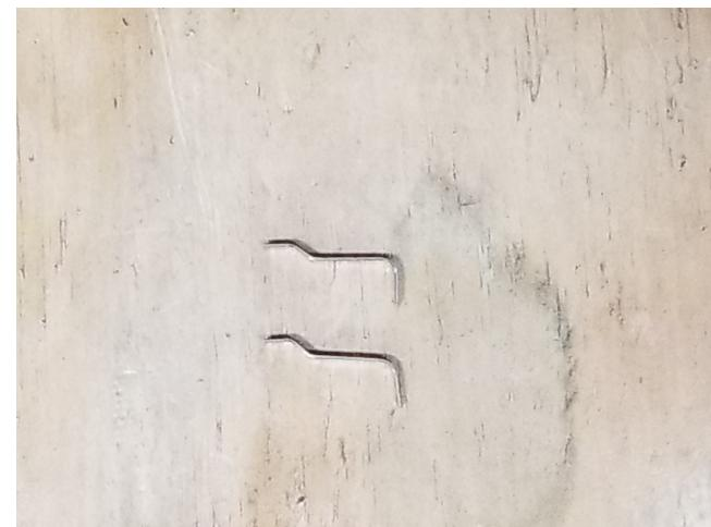
Adjust Barrel lock spring as shown. Top is OE, Bottom is adjusted.
