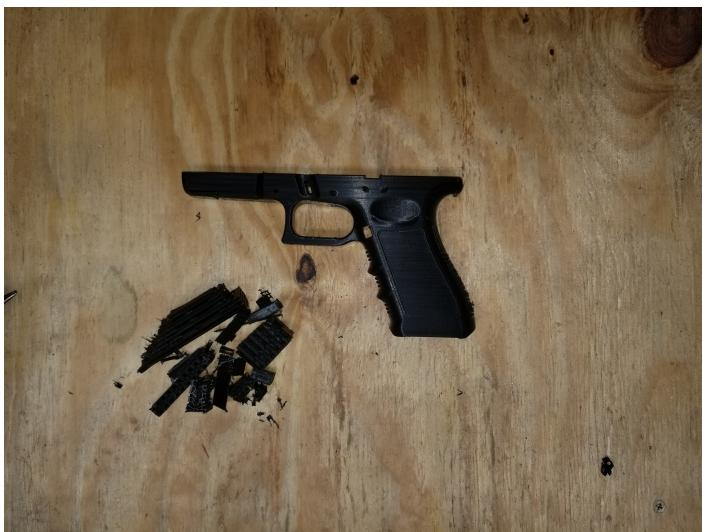
Remove rear supports, then remove supports from the front , working your way to the back. Make sure to remove any loose filament strands in the rail cavities. Once internal supports are removed, push out trigger guard supports.
