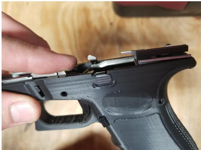
Install locking block, slide lock and trigger pin.
