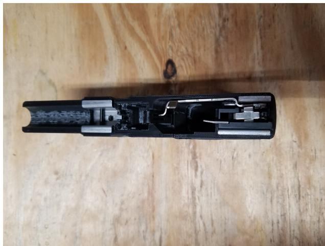
Install rear rail, trigger assembly and pin.
