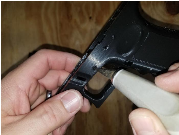
Use a sharp blade to lightly go around pin holes. Only remove material at opening. Check fit and remove more material as needed. Pins will fit snugly.
