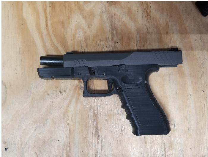
Make sure the slide moves freely with no binding. Check for proper trigger function. Rack slide several times with a decent amount of force. Insert an empty magazine and check slide lock function. Once everything works properly, use dummy rounds to check operation before firing.
