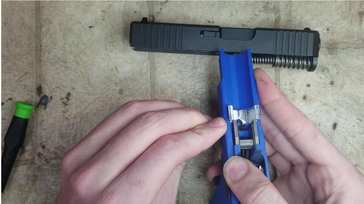
Pushing down spring with the latch
