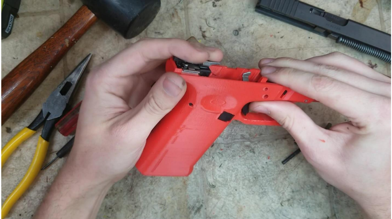
Pin fully installed. It should sit slightly recessed on both sides.
