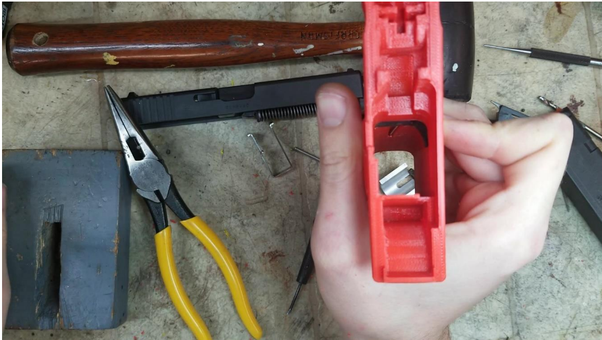
Spring snapped into the proper position after pushing it to the right
