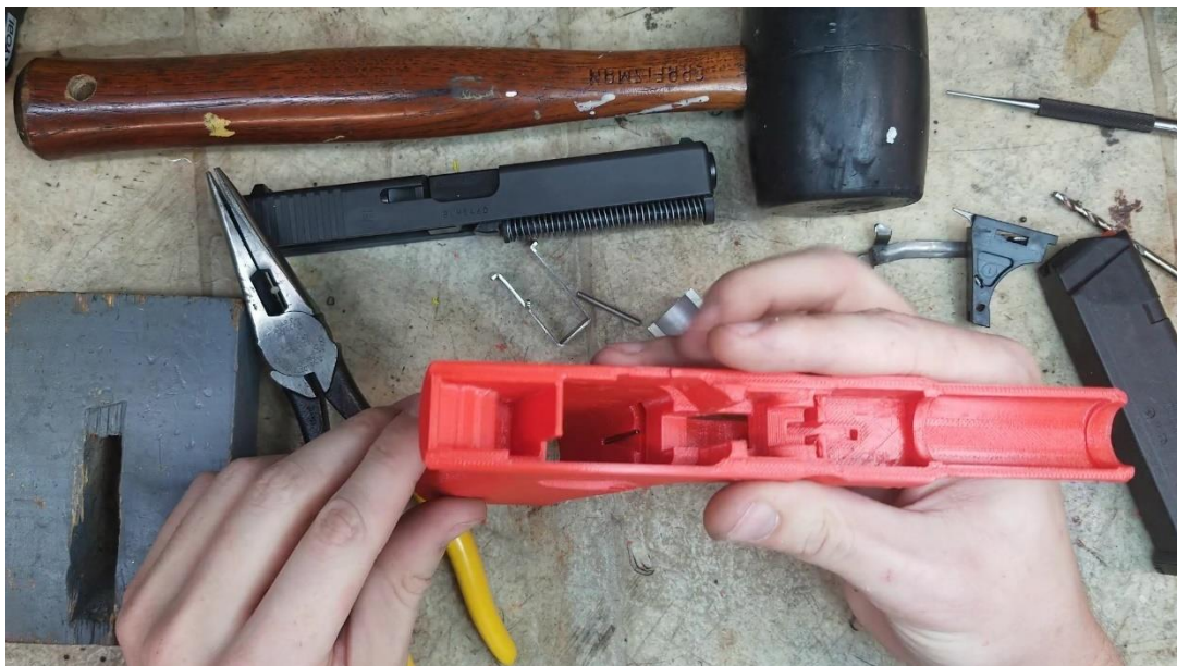
Mag catch spring fully inserted
