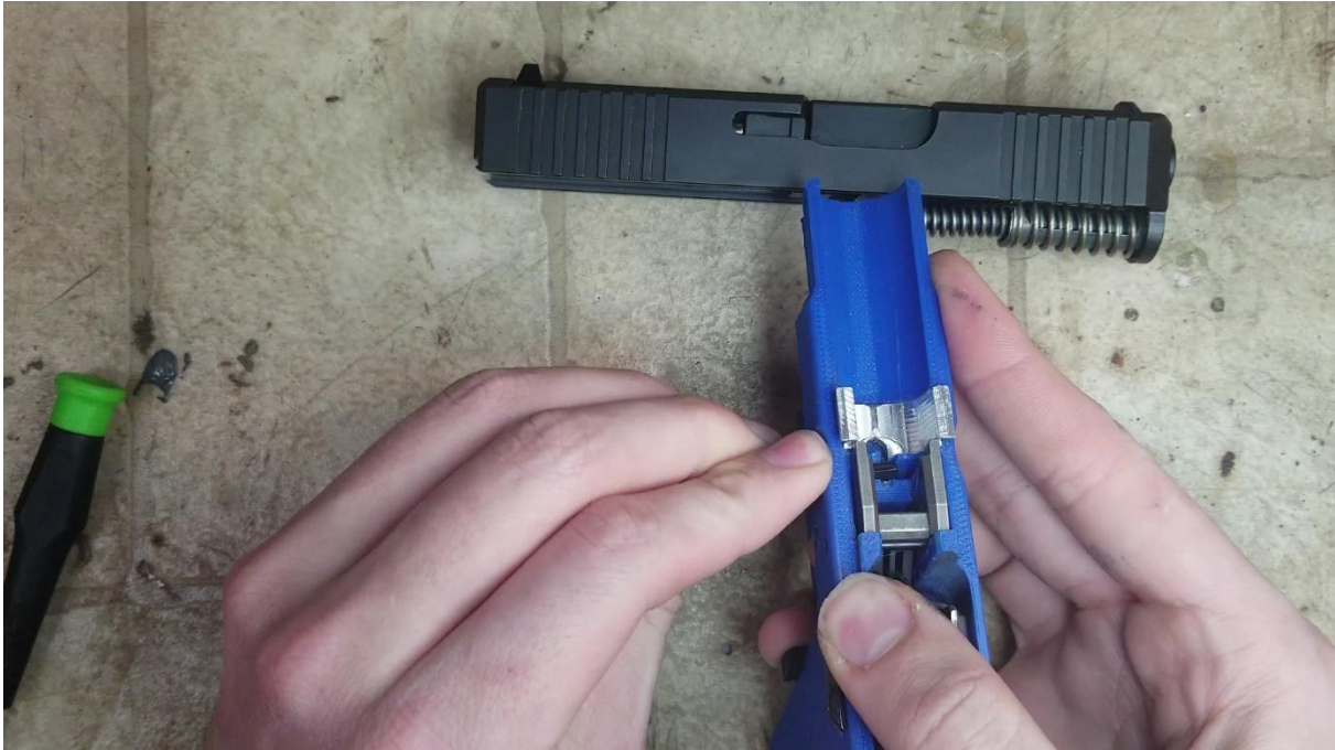
Pushing down spring with the latch
