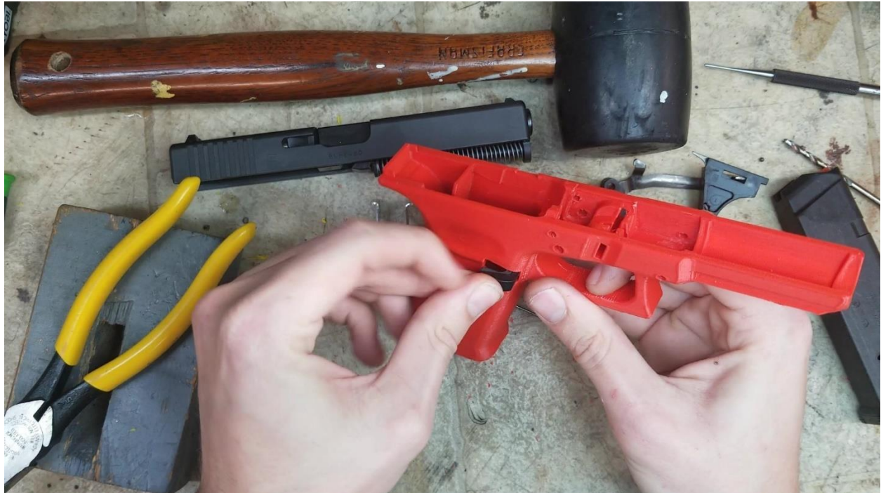
Test fitting the magazine catch
