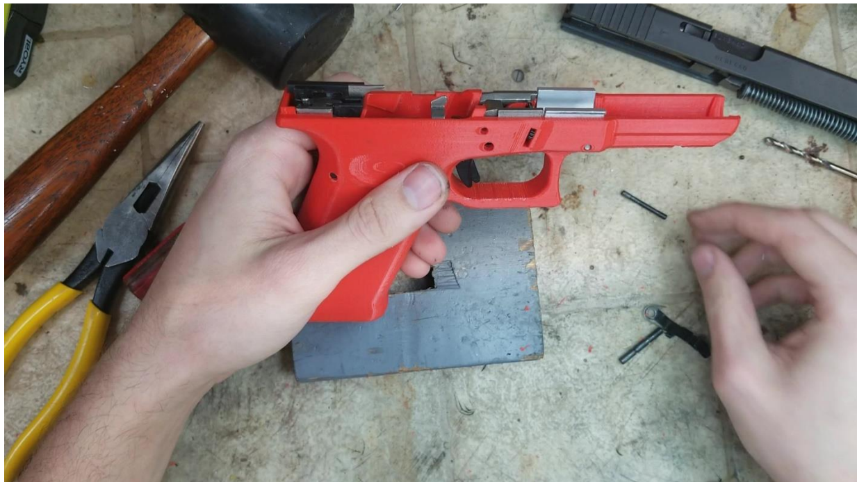
Locking block fully inserted.
