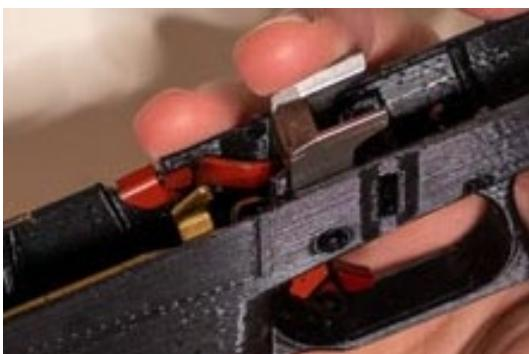
Place the locking block on top of top the trigger, ensuring that the trigger shoe and slide lock lever are in-between the “legs”.
