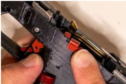
**TIP:** The pin will be correctly positioned when you hear a “click”, indicating that the slide lock has engaged the slot on the pin.
