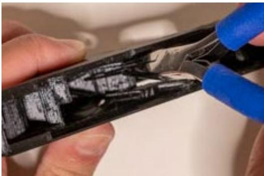
**Insert the magazine release spring into the slot in the magwell.**
