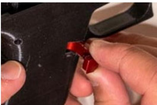
**Insert the magazine release, and ensure the spring secures into the slot on the release.**
