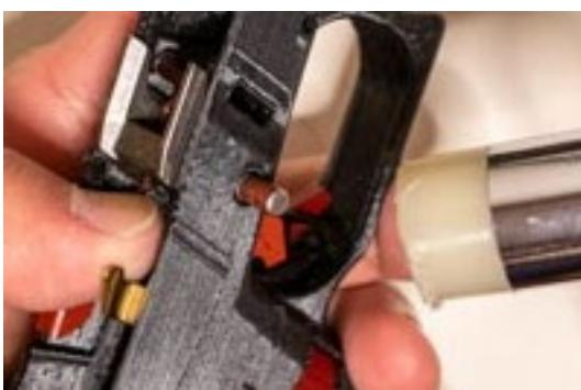
Install the trigger pin beginning on the righthand side of the frame.
