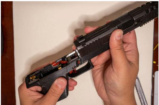
**Insert the slide onto the front rails.**
