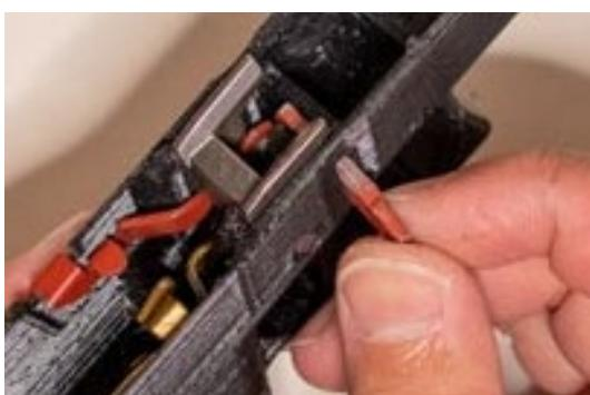
**Insert the slide lock at an upwards angle and use the slide lock to press down on the slide lock spring.**
