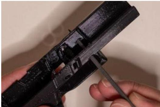
**Remove any debris from the openings on the frame.**
