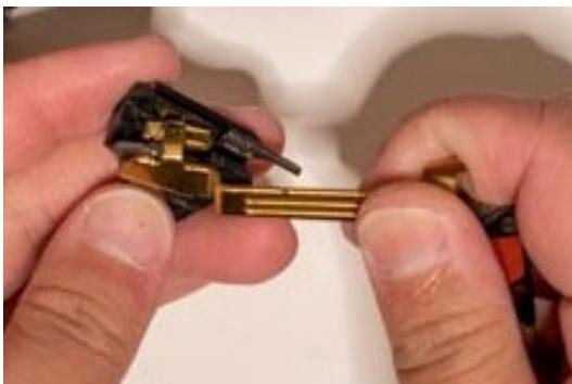
**Assemble the trigger housing and trigger bar.**
