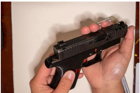
**Press the slide back onto the frame and slotted onto the rear rails.**
