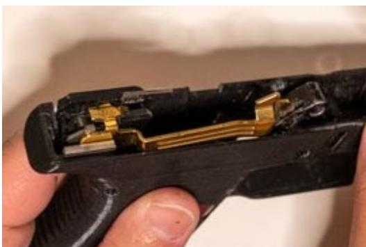
**Insert the trigger housing down between the rails, while ensuring the trigger clears the trigger hole.**
