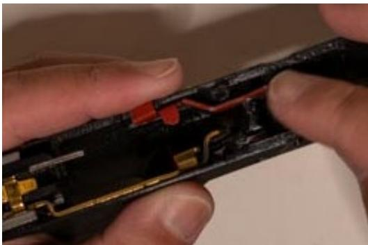
Insert the slide lock lever to the left of the trigger shoe.
