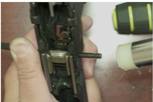
Insert the trigger pin on the side *without the notch* into the left side of the frame.
