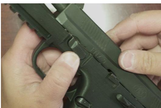
**Rack the slide back, and use the slide release lever to hold the action open.**
