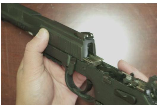
**Place the assembled slide onto the frame.**
