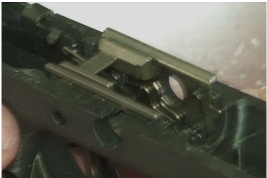
With the rails seated in place (they shouldn't move or rock back and forth), insert the slide lock lever from the front into the rear.
