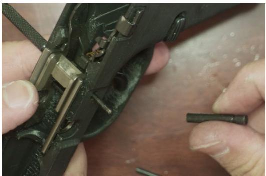
Use a punch to align the slide lock, trigger, and slide lock lever holes against the rails and frame.
