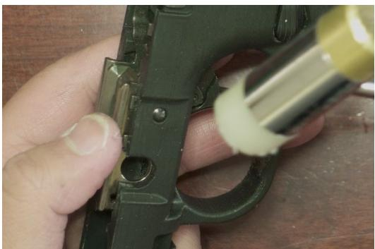
Tap the pin through the frame, ensuring it captures the rails, trigger, slide lock, and slide lock spring.
