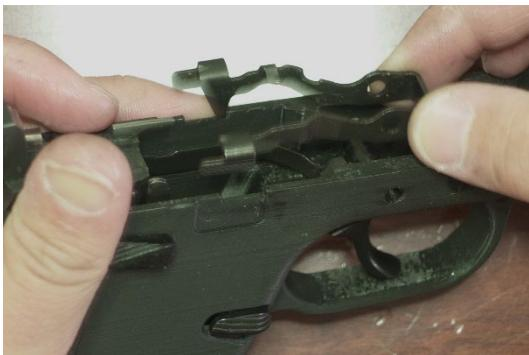
Place the slide release into the frame.
