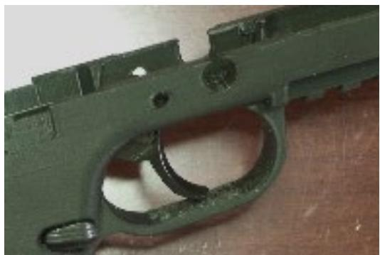
**Remove all supports. Chase out the trigger pin hole with a 4.0mm drill bit.**
