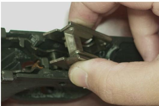
Pinch together the front rails and the unlock block. Begin to insert it into the frame.
