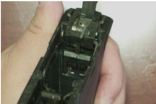
Ensure the fire-control unit is fully seated.
