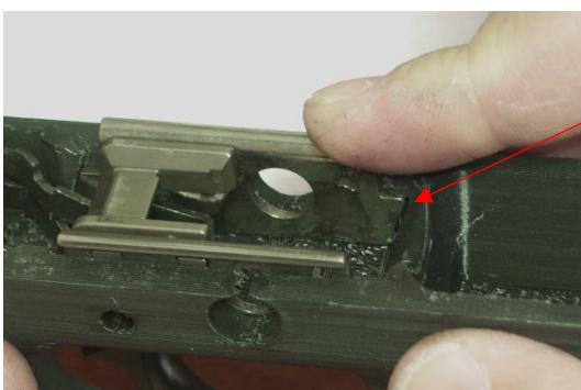
**IMPORTANT!** It is important to have the rails flush in the frame- there is a critical notch that ought not to be modified, as it is used to help retain the front rail.
