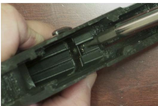
A properly installed spring should let you depress the button from either side without much resistance.
