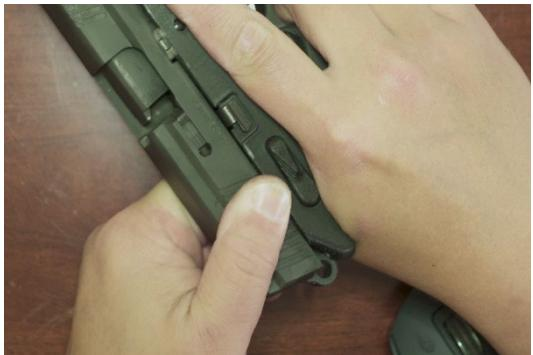
**Pull back on the slide to release the slide lock and return the gun to battery.**
