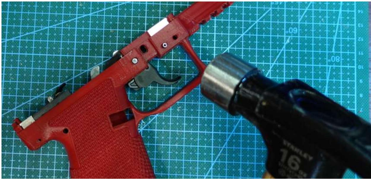
Use the precision tooth straightening tool to whack the 3mm pins into their respective orifices. Then, grab the locking element, its spring, and the small pin with a small nipple on each end.
