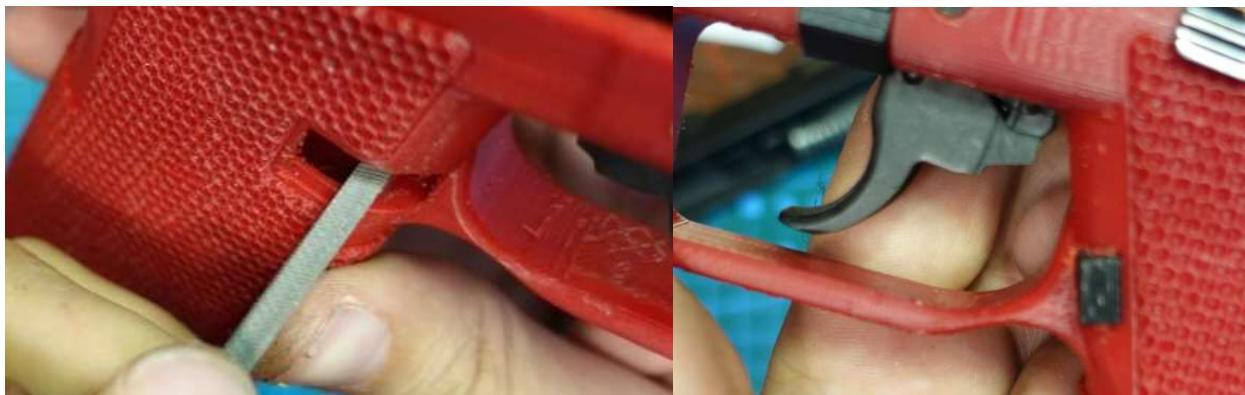
Next, install the magazine catch spring. Just drop it into the hole below the mag catch inside the grip.
