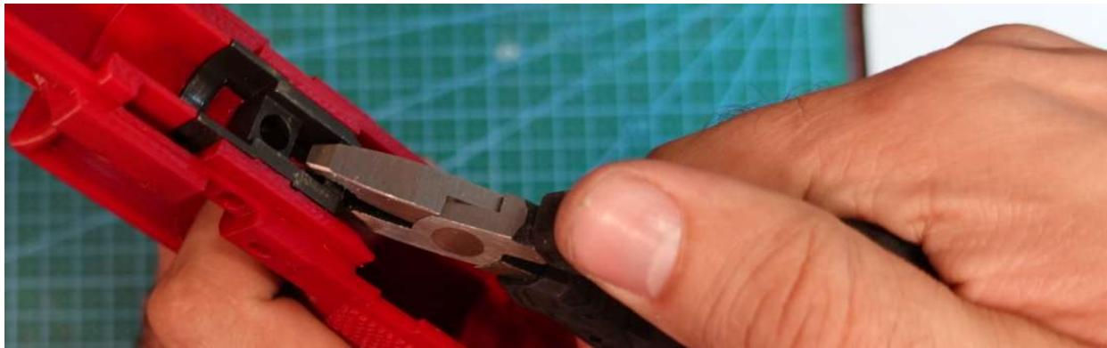
If you need to remove the locking block for additional fitting, carefully wiggle it out as shown. Once it is fit, remove the locking block and set aside.
