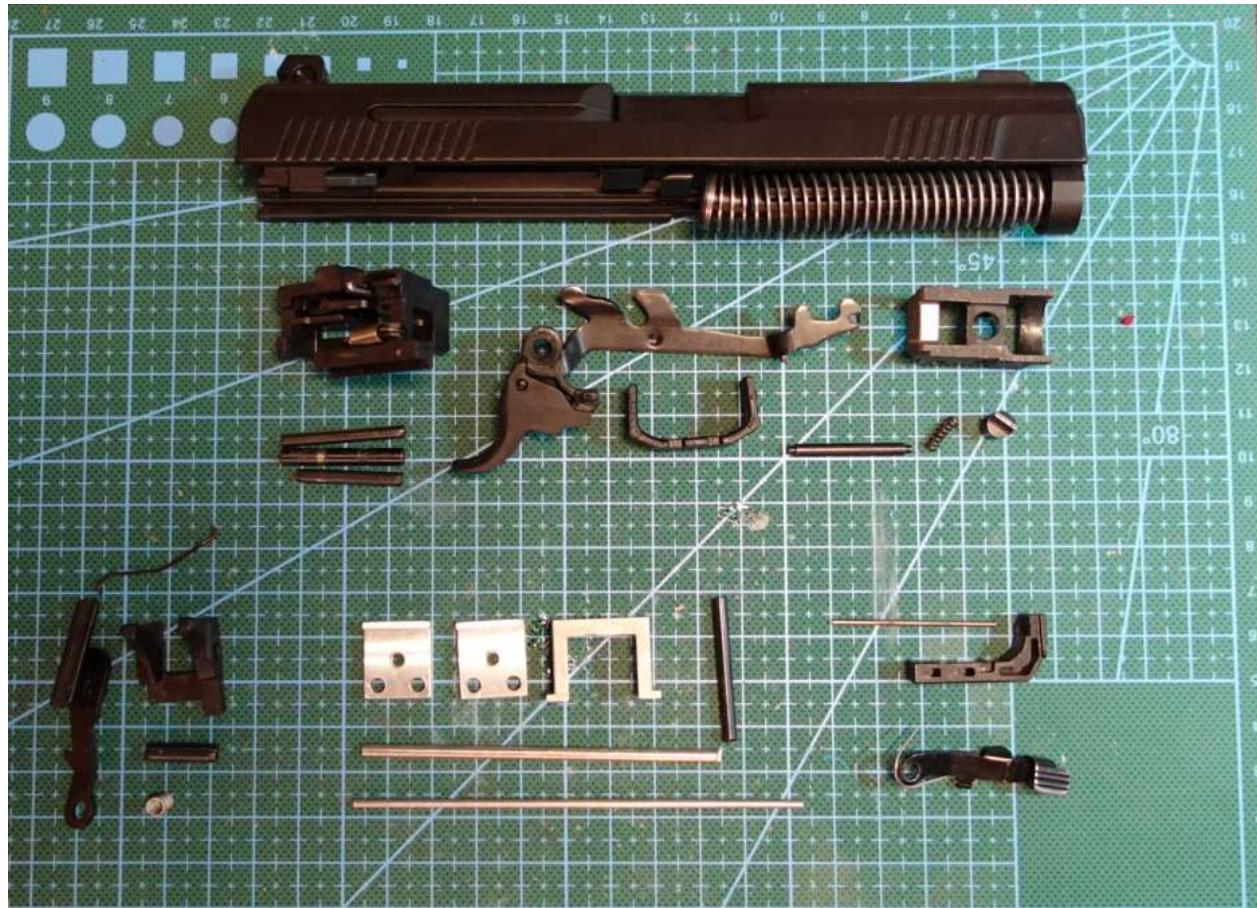
The parts in the bottom left corner of the above image are those from the original kit which will not be used. Those are the slide release and spring, magazine catch, magazine catch pin, and magazine catch spring.
