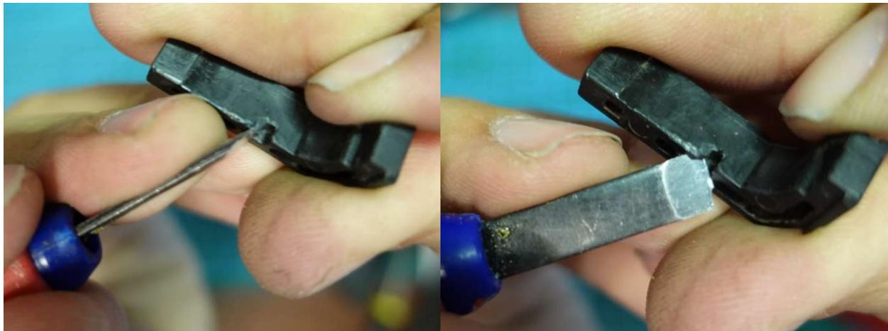
Insert that mag catch, push it past the spring, then use a tool to push the spring over into the notch we just enlarged.
