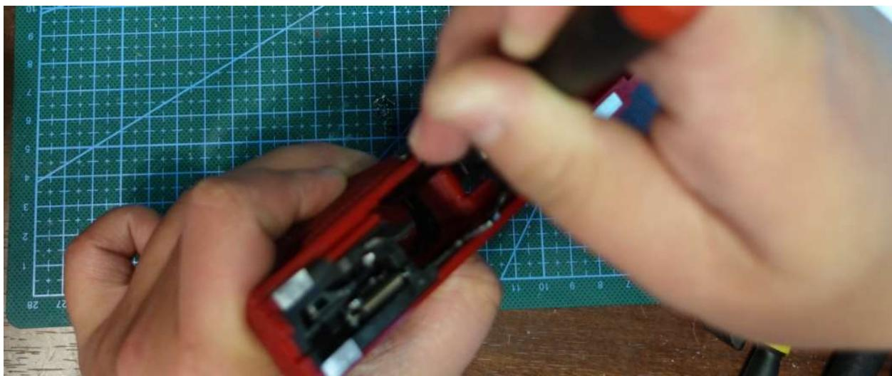
The frame is now assembled. You may need to do some final fitting on the rails, or you can just cycle the action repeatedly until the steel slide wears into the aluminum rails. I've done it both ways, and both frames have held up tremendously.
