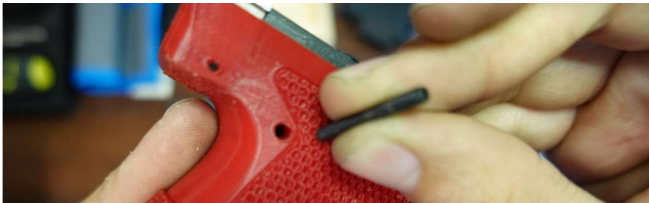
The shorter 3mm pin retains the trigger pack. Whack this sucker in and do your best to center it. Then, depending on what you're using for a rear pin, either grab the 2mm coil pin, or 2mm stock. I like using fairly soft rear stock to effectively rivet the rear rail in place.
