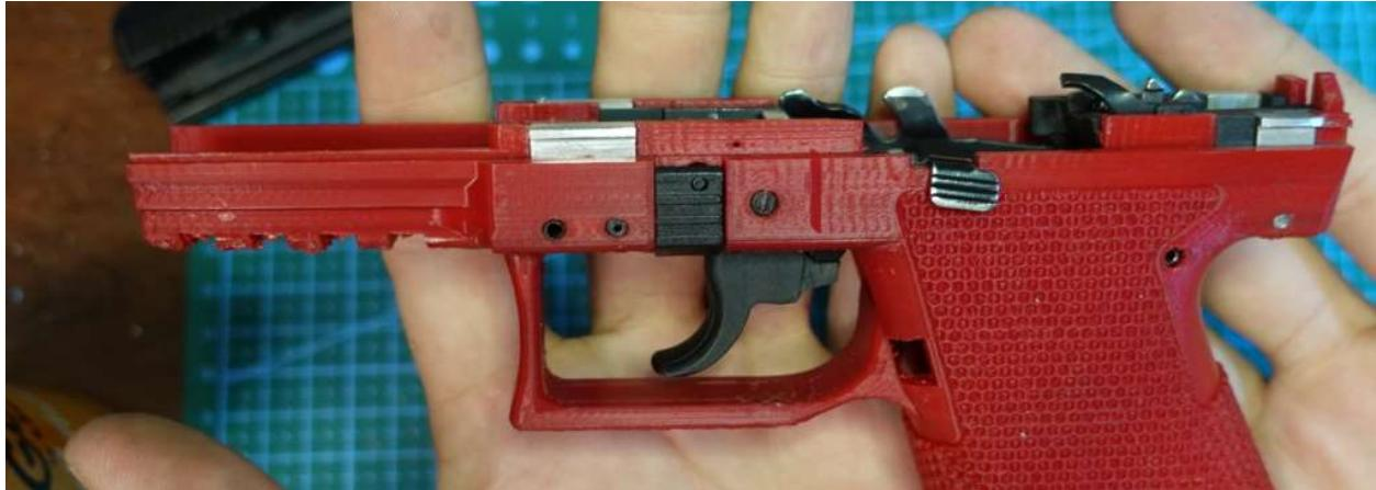
Now we prepare for the mag catch by cleaning out the mag catch area. Use a little file or whatever. Test the fit with just the mag catch. Make sure it's smooth.
