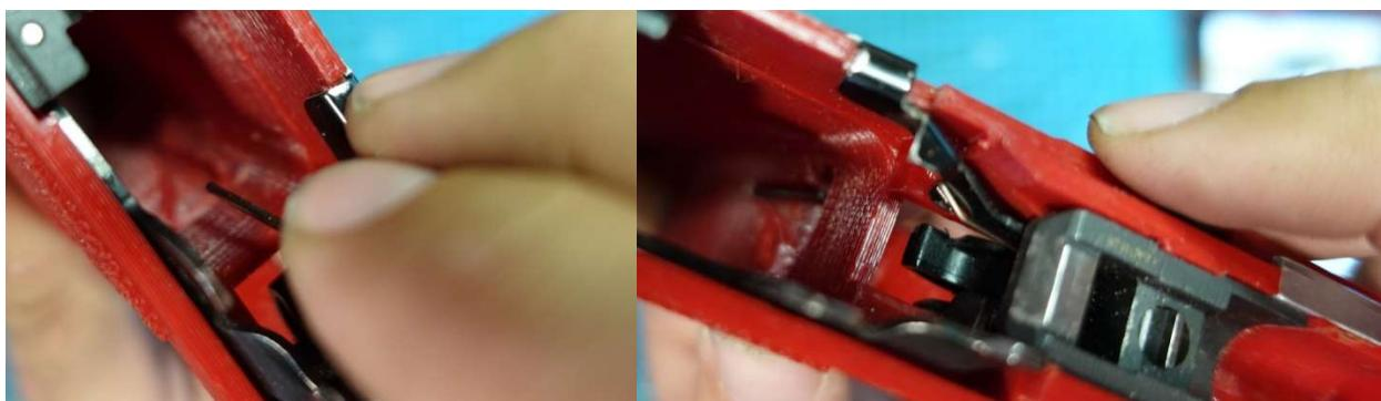
I recommend doing a slight modification to the magazine catch to make installing the spring just that little bit easier. Cut a small angle into the area shown below.
