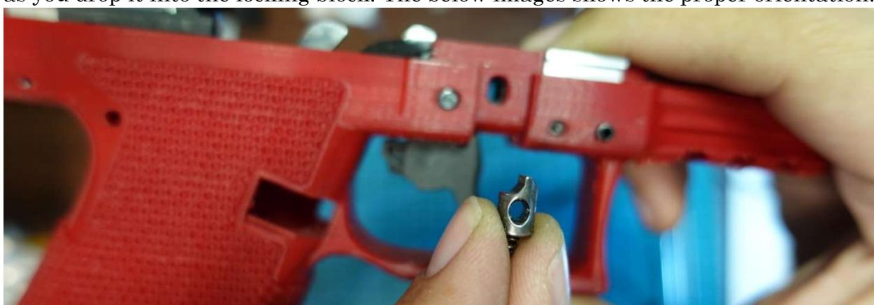
Place the pingle, springle into the large hole on top of the frame, the hole through which the ovoid shape is cut on either side, and keep pressure on the shaped locking piece. This is the track your disassembly lever sits in. The small, nippily pin will secure the pingle, springle, and lever.
