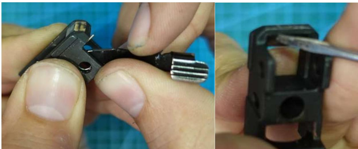
Observe how the G17 slide catch and spring interact with the locking block. (above, left) We need a notch to capture that spring, and we will put that notch in the spot indicated. (above, right)
