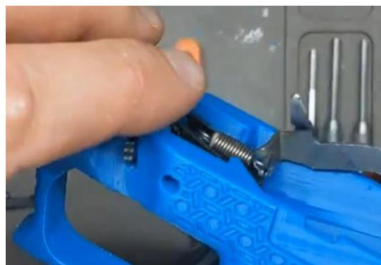
**Step 8:** Install Locking Block, which will now capture the trigger assembly in place.
