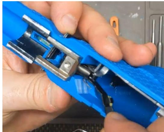
**Step 10:** Install Trigger Pin. Note the notch orientation and install as shown from the right-hand side of the frame.
