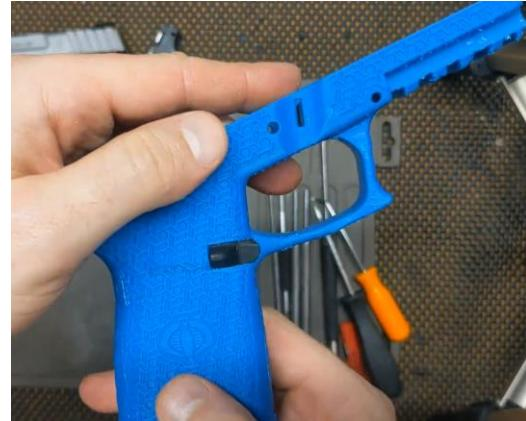
**Step 2:** Install the Magazine Release Spring. Make sure the fat end goes in towards the bottom of the grip. Insert from the top using long needle-nose pliers.
