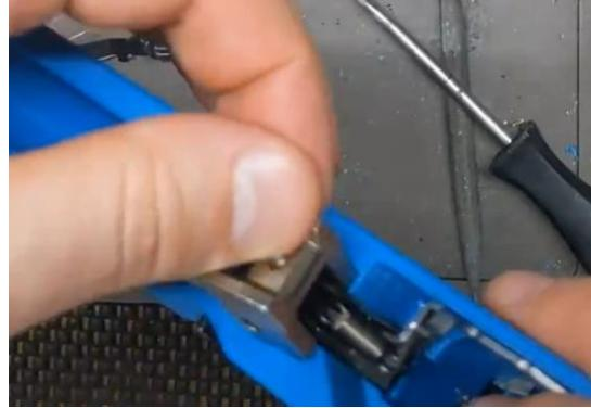
**Step 9:** Install Slide Catch Lever. Slide in to the notch on the lefthand side of the trigger.
