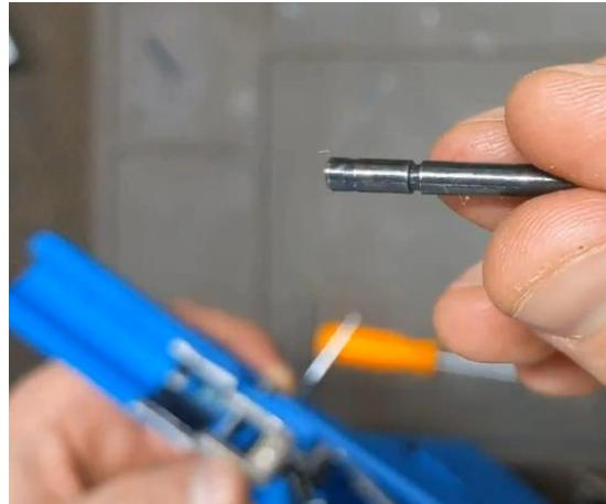
**Step 11:** Install Rear Sear Housing. For the SD40, the rear rails are part of this housing. Visually check hole alignment where the rear pin will go.
