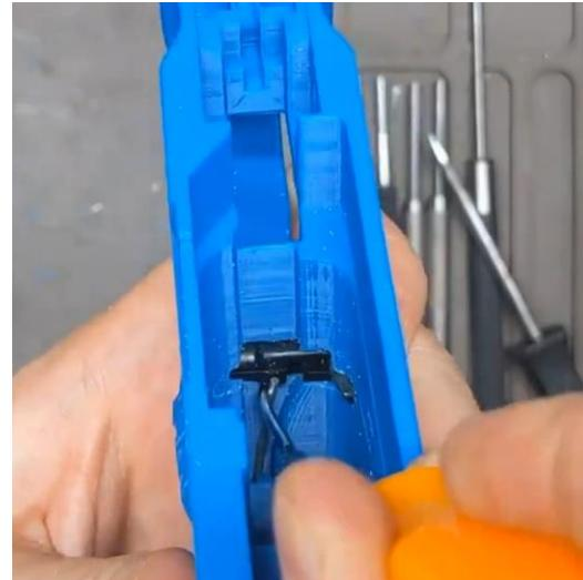
**Step 4:** Test Magazine Retention and Ejection. Grab a magazine, make sure it locks in and ejects freely.
