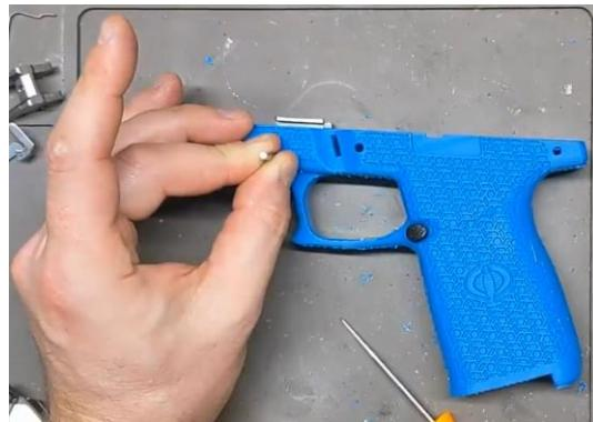
**Step 6:** Install Takedown Bar and Spring. First, insert the spring into the pocket. The straight section goes into the pocket. Depressing the spring with a screwdriver, slide the takedown bar thru the slots in the frame.
