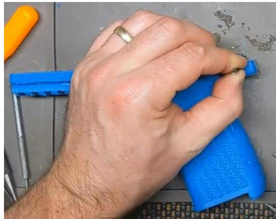
**Step 14:** Assemble Slide to Frame
