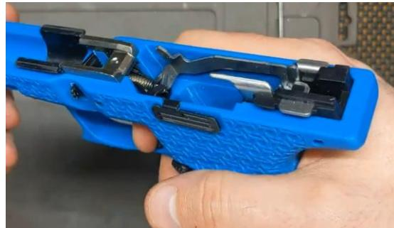
**Step 13:** Install Sear Housing Roll Pin.
