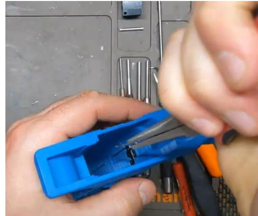
**Step 3:** Install the Magazine Release Button. Using a pick or hook, pull the mag release spring into its slot in the mag release button.
