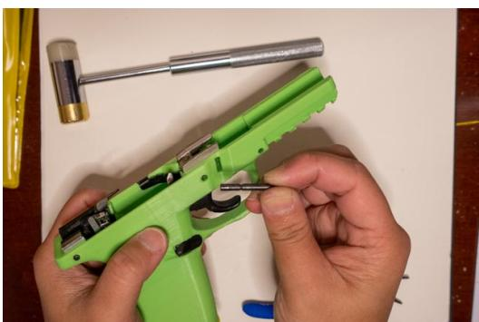
**Using the trigger pin, pin the locking block, trigger, trigger return spring, and slide lock in place.**
