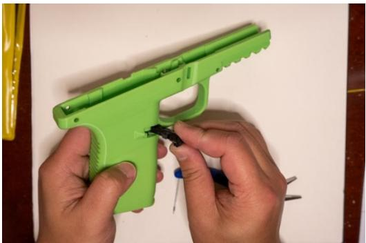
**Using a flathead screwdriver, navigate the spring into the pocket of the magazine release button.**
