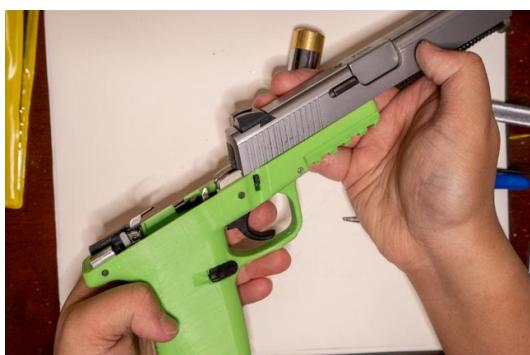
**Place the slide assembly onto the frame.**
