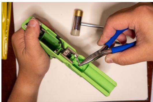
Place the straight end of the takedown lever spring into the recess in the front of the frame.
