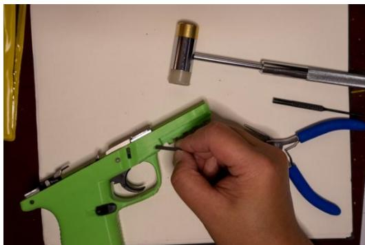
**Pin the front rail block into place.**
