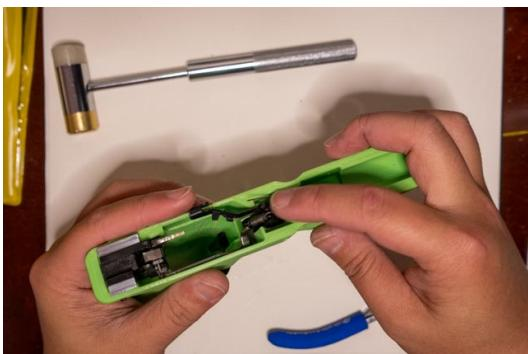
**Place the slide lock to the left of the trigger.**
