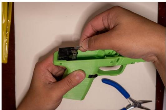
**Insert the rear fire control module.**
