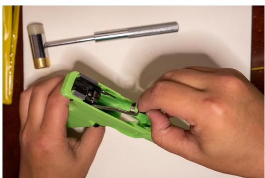
**Insert the “hook” of the trigger bar up and into the fire control module.**
