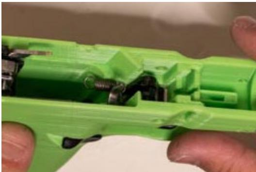
**Disengage the shoe safety and slip the trigger through the hole in the frame.**
