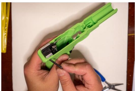
**Pin the rails and rear fire control module in place.**
