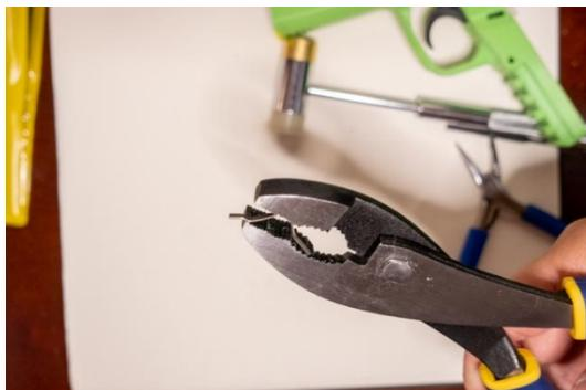
**(SW9 ONLY)** Flatten out the takedown lever spring, but not completely.
