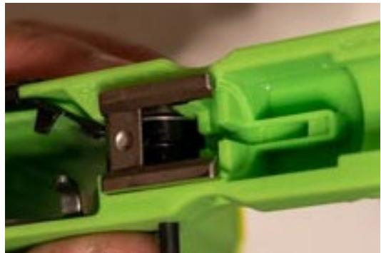
It may be helpful to use a punch to keep the trigger return spring taut as you push the trigger pin through.
