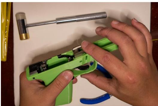
**Insert the locking block on top of the slide lock and trigger.**
