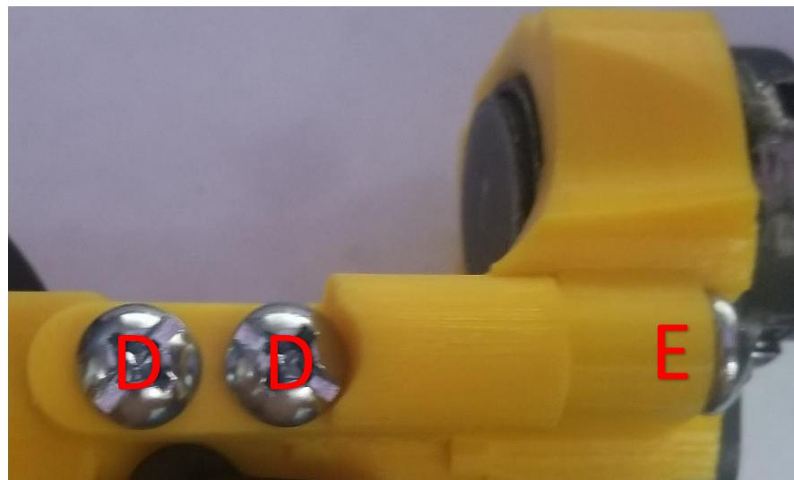
Before starting this step, it is very important that you extend both take down pins. Then install the Buffer to FCG Left piece using the appropriate screws to fasten the reinforcement piece. The screws should be tight to fasten, as designed, so use some force to tighten them in. Once fastened, attach the entire AR Upper Receiver and close the takedown pins. The pins may have difficulty closing due to tight fitting.
