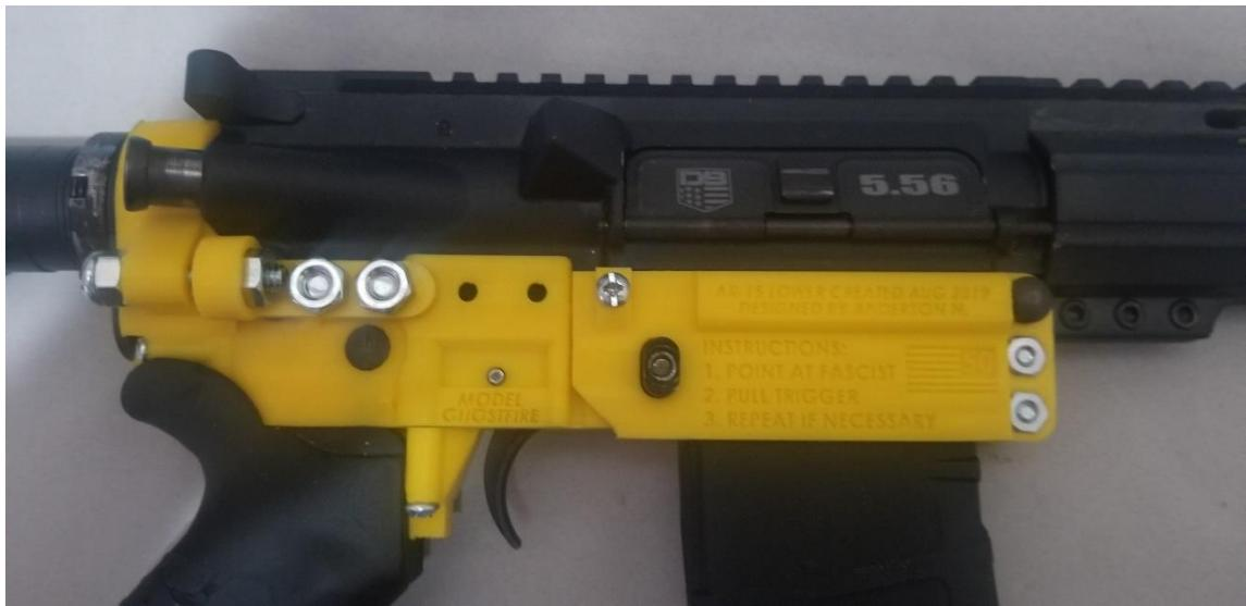
This test involved 40rnds of American Eagle 55Grain 5.56 NATO Full Metal Jacket. The test proved a breakthrough: The weapon was expected to explode around the buffer tower, but it did not. The weapon performed without major malfunction except one
