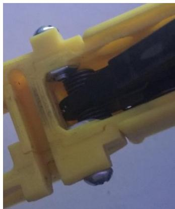
This is what it should look like when the screw and nut are added. Make certain that the hammer does not touch or contact the screw and nut when cocked and dry fired. Remember to brace the hammer when the trigger is pulled.
