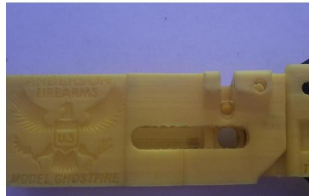
Start adding the Magazine Well to the Fire Control Group By sliding the Fire Control Group vertically into the Magazine Well. Little force may be required to fully connect the two main pieces and an audible snap may be hear once fully attached, which should not be mistaken as cracks or damages. Although the picture does not show the washer from the previous step, it should still be on the Fire Control Group when attaching the Magazine Well.
