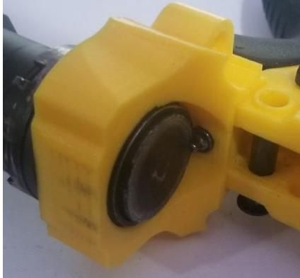
Now install the buffer tube and tighten the castle nut. In this step it is ok to tighten the castle nut with force, as you would normally do with a normal lower. Tighten it to where the castle nut will not come loose when firing.
