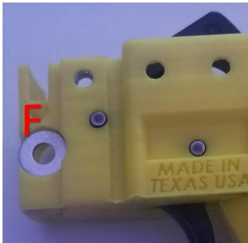
This step is important: add the washer indicated. This washer allows the magazine release spring to be installed correctly.
