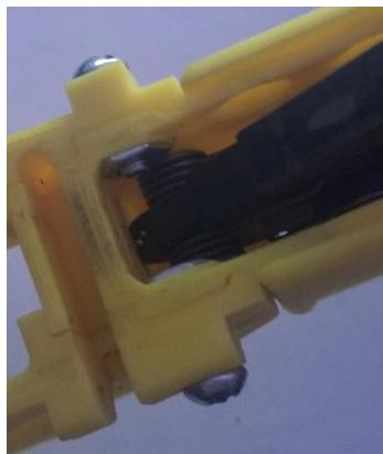
This is what it should look like when the screw and nut are added. Make certain that the hammer does not touch or contact the screw and nut when cocked and dry fired. Remember to brace the hammer when the trigger is pulled.
