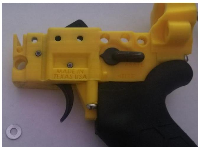
In this step, the grip and the fire selector are added. Observe how the grip sits against the buffer tower. It is important to install the buffer tower before the pistol grip. Fasten the Pistol Grip using the pistol grip screw.
