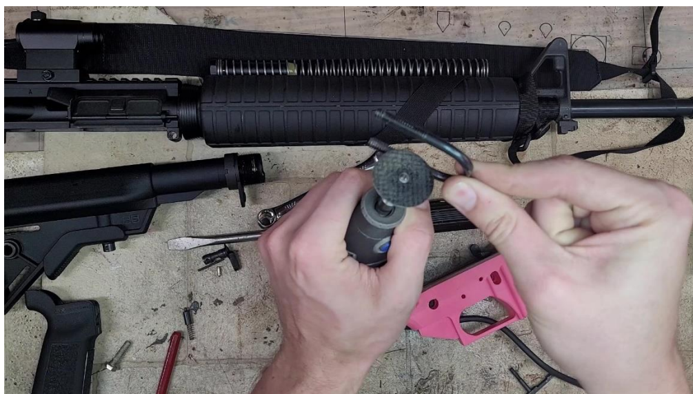
Example technique to grind down on the insides of the bolt using a Dremel tool – you will want to hold the bolt using pliers or a vice, as it will get too hot to hold quickly.
