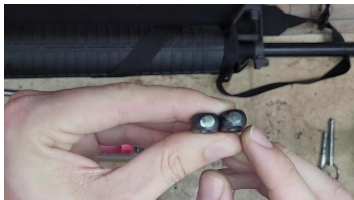
Grind down on the top of the eye bolts about this much – you want the top of the eye bolts to sit flush with the top deck of the lower.
