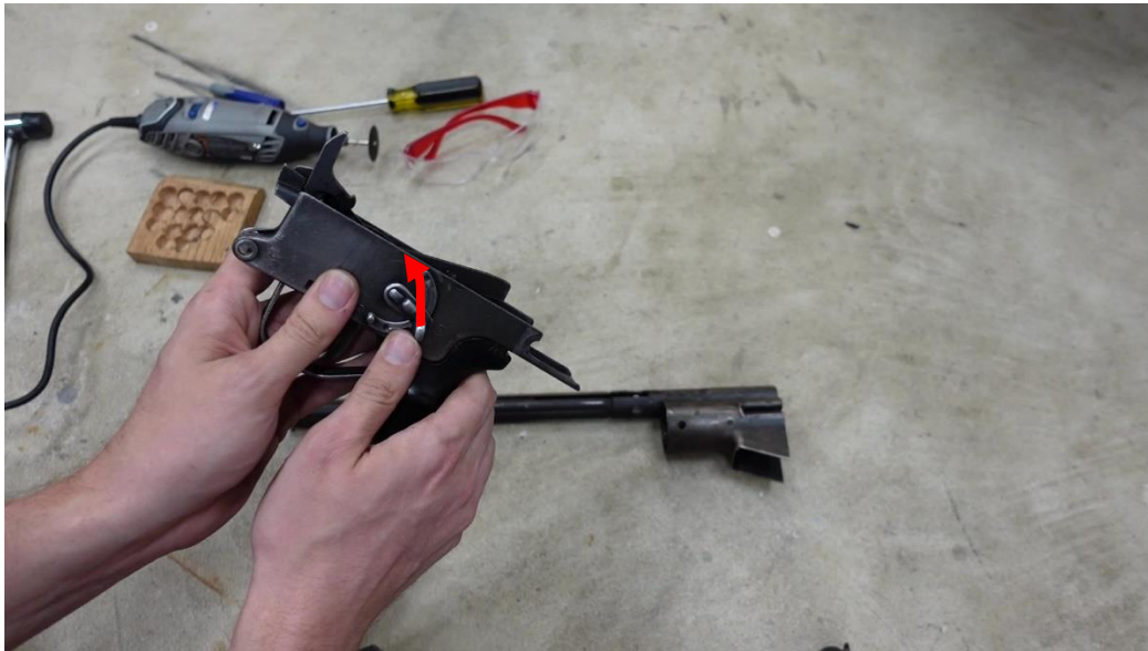
Rotate the selector upwards
