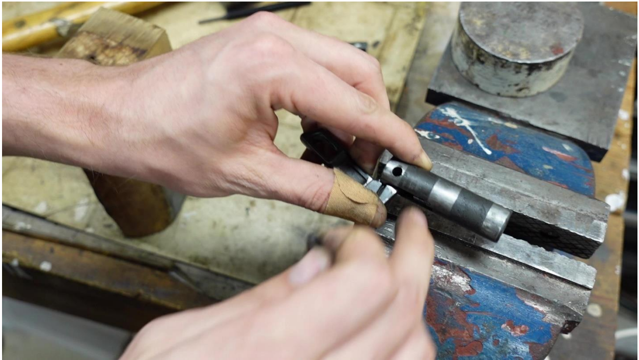
Line up the pin hole
