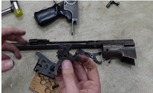
Take your trigger and disconnecter chassis.
