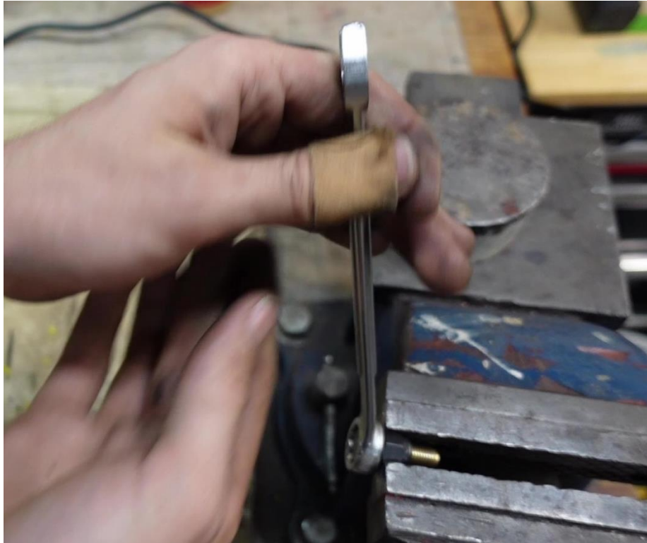
Thread the bolt fully into the locking nut.
