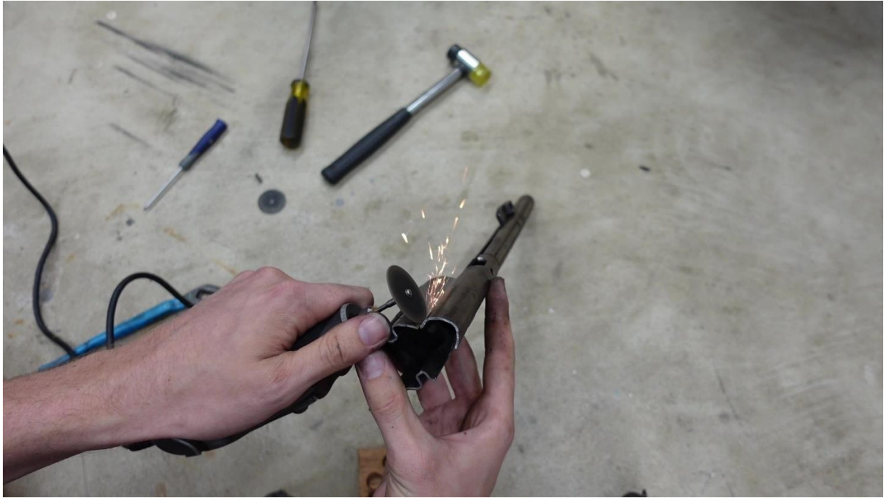
Cutting on the left side of the tube.
