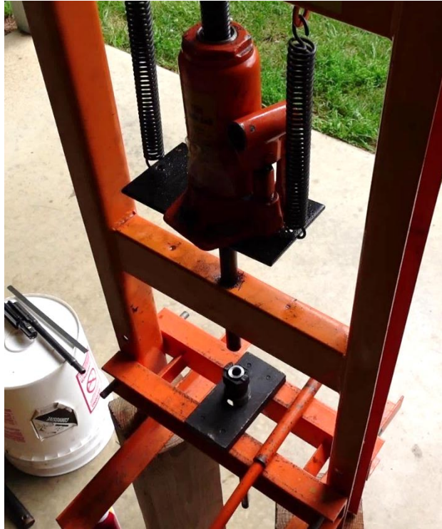
Place the barrel and trunnion together under the press ram.
