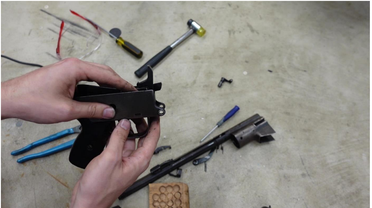
Set the trigger housing back into the grip assembly.
