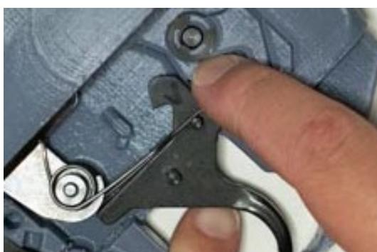
**Place the arms of the spring on the spring retention pin on the trigger.**
