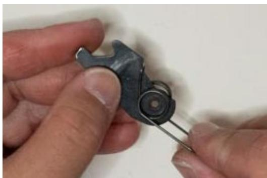
**Align the hammer/trigger spring onto the hammer.**
