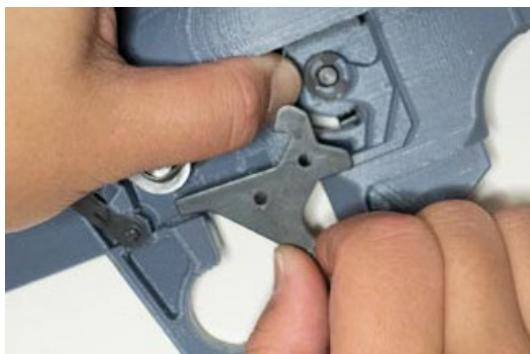
**Using your thumb, lift both arms of the spring upwards.**
