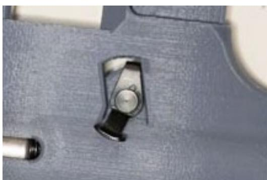
Place the safety through the hole, resting on the detent ball.
