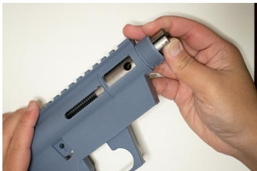
**Insert the bolt assembly into the receiver, with the charging arm hole facing the right-hand side.**
