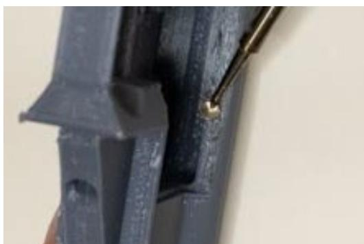
A soldering iron can help smoothen and remove stringing from the receiver.
