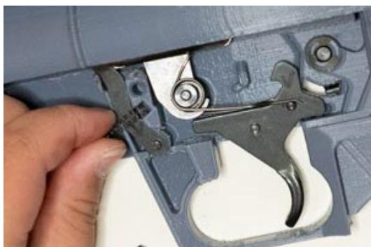
Place the magazine release spring into the slot.
