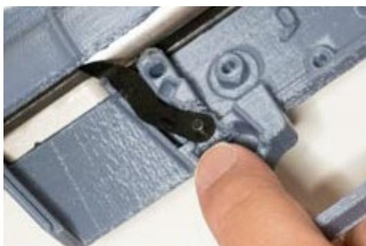
Once the hole of the ejector is aligned, use the magazine release pin to secure it in place.
