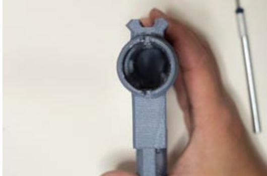
**Remove any debris or support material from the frame.**
