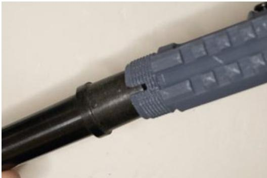
**Insert the barrel into the receiver, with the notch on the barrel engaging the receiver.**
