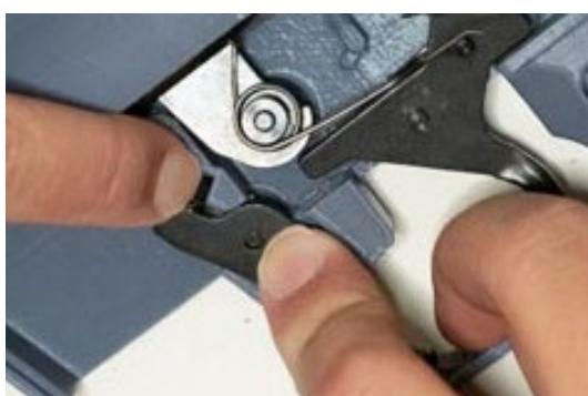
While holding down the magazine release spring (to keep it from flying away), install the magazine release. Do not let go of the spring.
