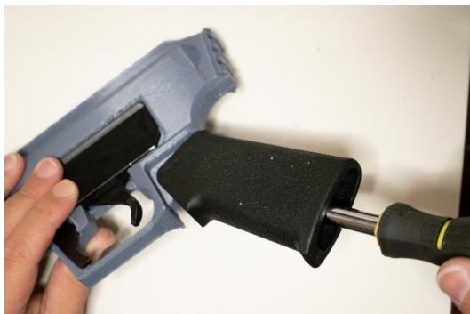
Install the AR-15 grip by placing it on the receiver and screwing it in.
