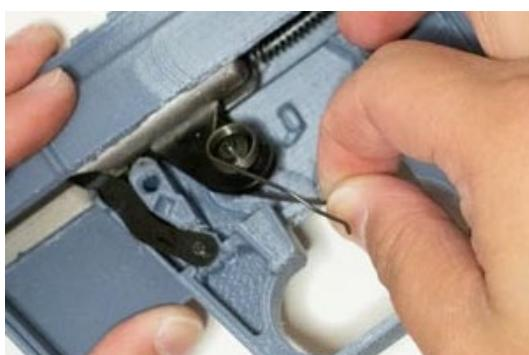
**Insert the hammer up into the bolt.**
