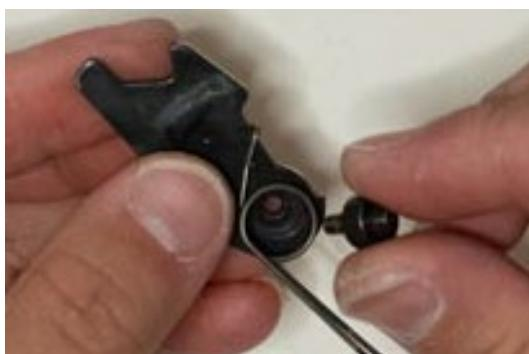
**Place the hammer retention pin on the left-hand side of the hammer**
