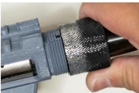
**Use the barrel nut to secure the barrel to the receiver.**
