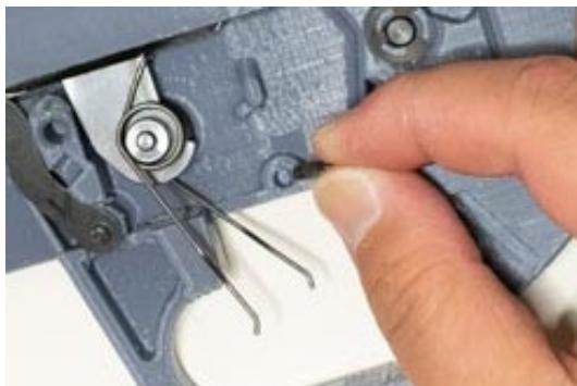
**Insert the trigger pivot pin.**
