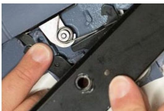
Place the housing plate over the assembly. Only remove your finger from the spring after the plate is over it.
