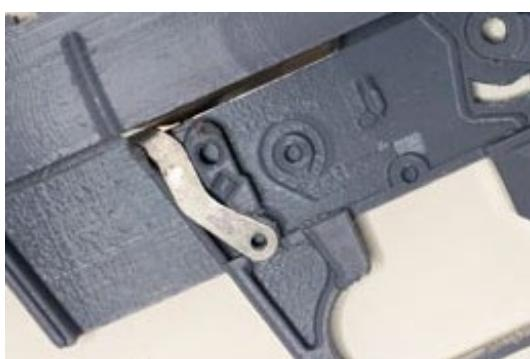
Getting the ejector into the slit machined out on the bolt is essential.
