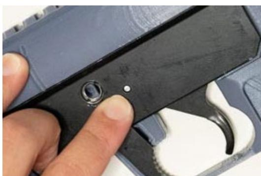
Align the plate so it interfaces with the hammer pin...
