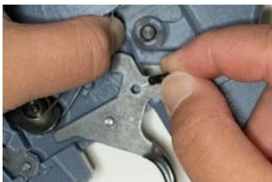
**While still holding the arms of the spring, insert the spring retention pin into the trigger.**
