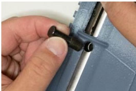
**Insert the charging arm into the bolt to secure it to the receiver.**
