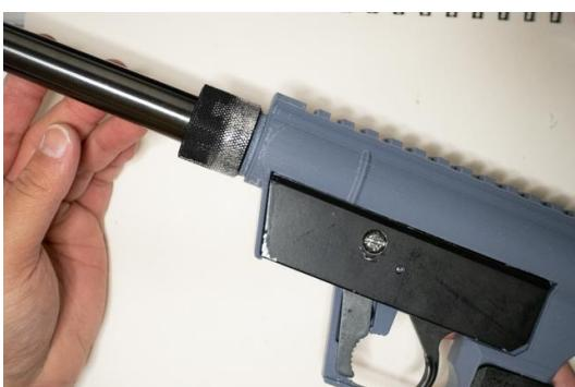
**Tighten the nut so that it holds the barrel snugly in place.**
