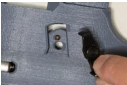
Place the detent ball onto the detent.
