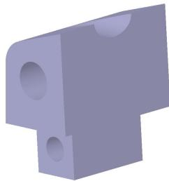
.22lr snap cap: print out and load in spent cases. Handy for function testing.
