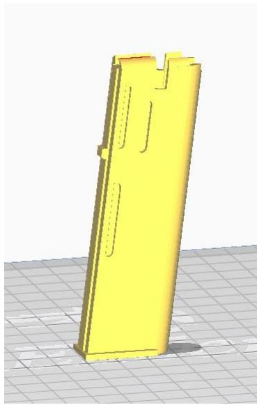
Follower, back flat side on bed (slicer should load it correctly)
