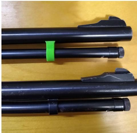
Barrel test print: Use this to practice sanding for barrel fitment, pin insertion...etc
