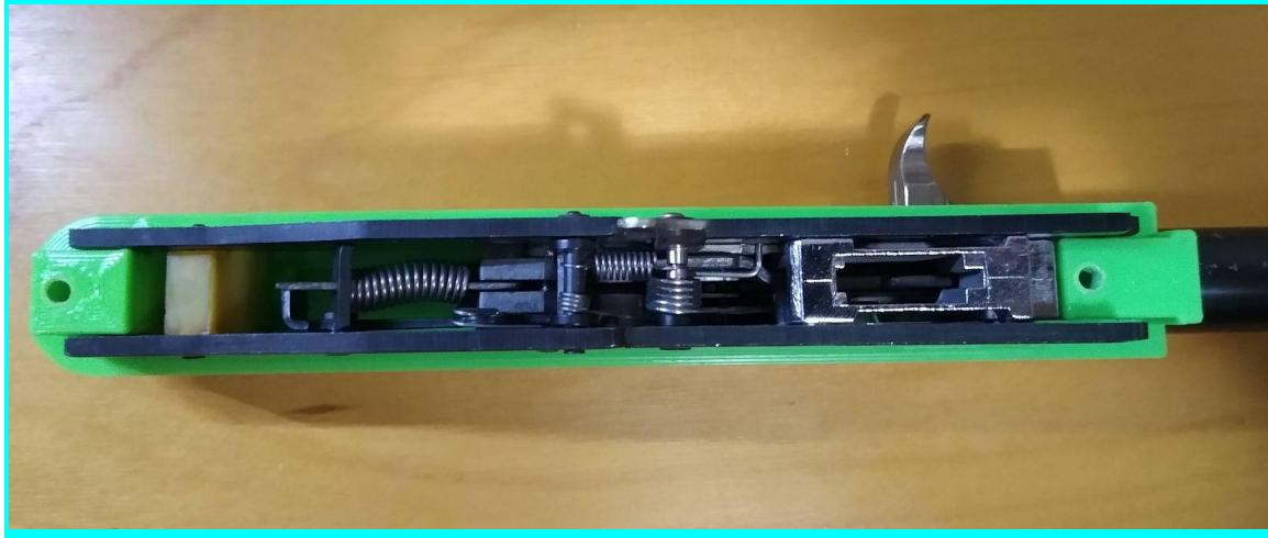
At this point you should be ready to drop it in the stock. Front and rear action to stock screws are self tapping.
