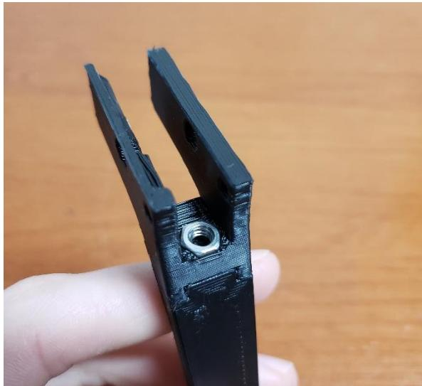
Next place the M4 nut in the corresponding spot on the frame. (This is a cut down demo piece to show where it goes)
