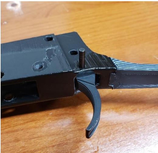
Insert the trigger pin.
