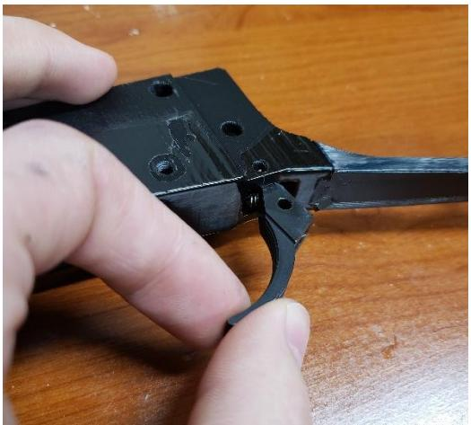
Put the trigger and spring into the frame. The spring should fit into the corresponding hole on the inside of the frame.
