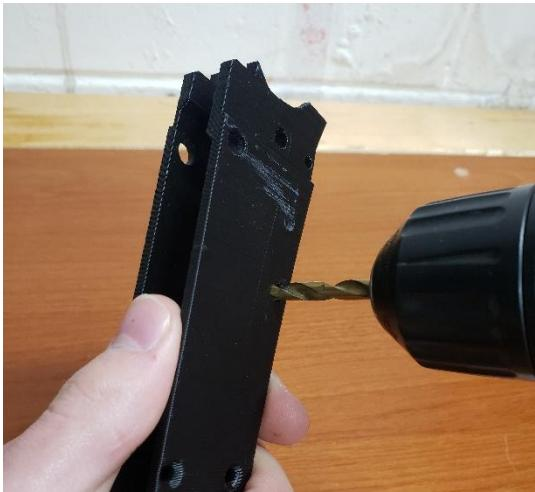
Use the same 13/64" (5mm) bit for the lever pin hole.
