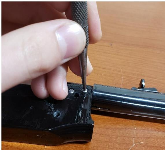
Carefully hammer your pins into place. This shouldn't require a ton of force.
