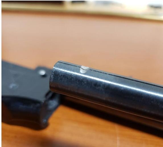
Install your mag tube. Make sure this notch goes up towards the barrel when installing.
