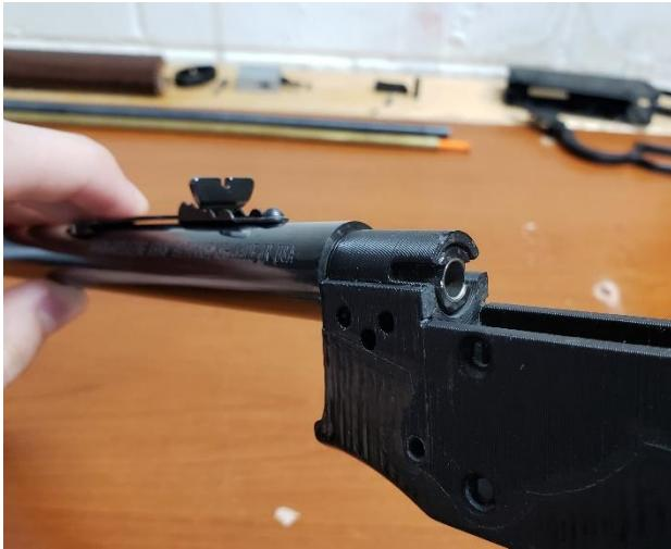
Insert your barrel into the frame. It should be tight, so rotating it while installing may help this go easier. Don't force it.
