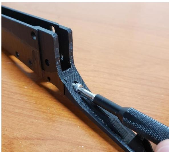
Connect the two parts with the M4 x 8 screw.
