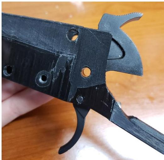
Line up your hammer in the frame and put in the corresponding pin.
