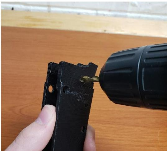
Take a 13/64" (5mm) bit to the hammer pin hole as shown.
