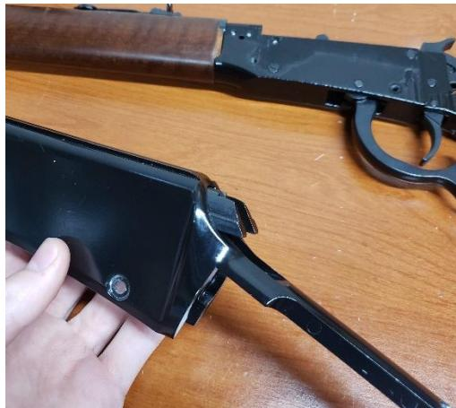
Slide the bolt into the top cover making sure to leave some of it out like this.
