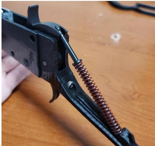
Rest your spring and guide assembly in the hammer like this.
