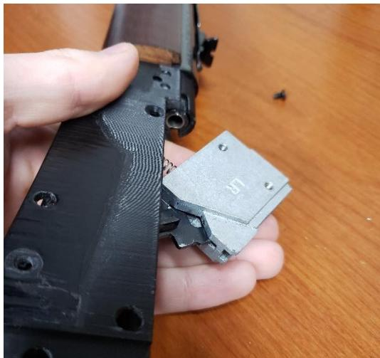
Flip the frame upside down and slide the carrier into place. Make sure the spring and plunger go underneath the carrier feed lever.
