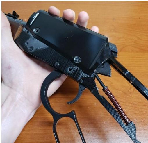
Open the lever partially and slide the cover and bolt onto the receiver. This can be tricky.
