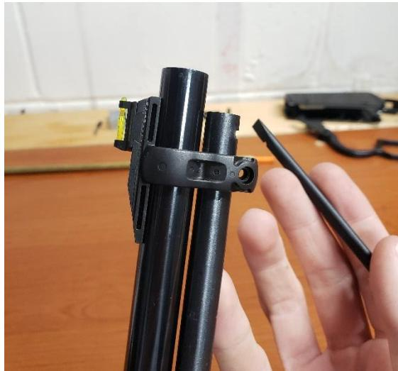
Remove the spreading tool and install the clamp screw. Reinstall your sight hood if taken off.
