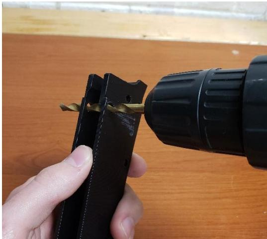
Chase each hole with the proper size drill bit. This makes assembly easier and helps prevent cracking. Take caution not to oval the holes.
