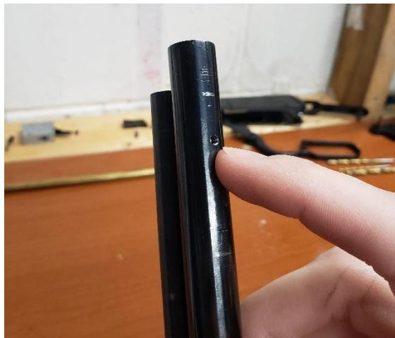
Note the threaded hole in the barrel. This needs to line up with your front sight.
