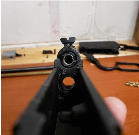
Check your barrel alignment often as you do this because it tends to rotate when installing the pins. Usually it can be twisted back by hand before you put the pins in completely. This may take a couple tries to get right.
