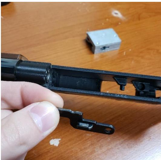
Take the carrier feed lever and install it into the frame. It should rotate freely. Some cleanup may be required in order for it to fit.
