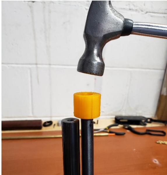
The mag tube should be a relatively tight fit. Make sure it is aligned and tap it into place using a piece of scrap material.
