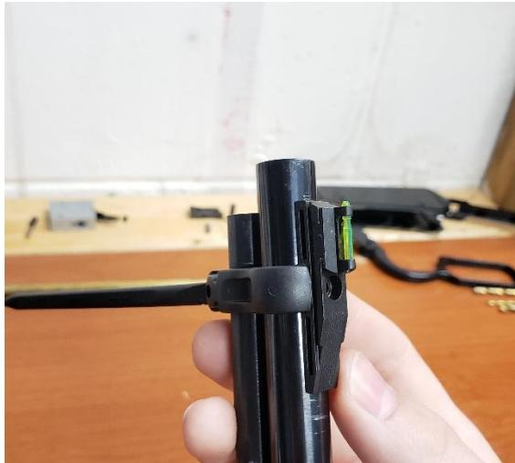
Slide your front sight onto the barrel and mag tube. Line up the sight and install the top screw.
