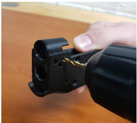
Sometimes it helps to carefully ream the taper pin holes out with the 1/8" (3mm) bit as well.
