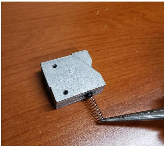
Put the carrier spring and plunger into the carrier as shown. Set this aside for now.
