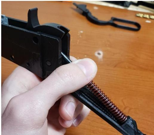
Press the guide rod down with your thumb. The guide rod should slide into the tang.
