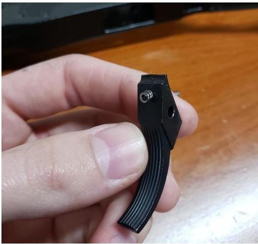
Insert your trigger spring into the hole in the trigger. It may help to put some grease on the spring to hold it in.
