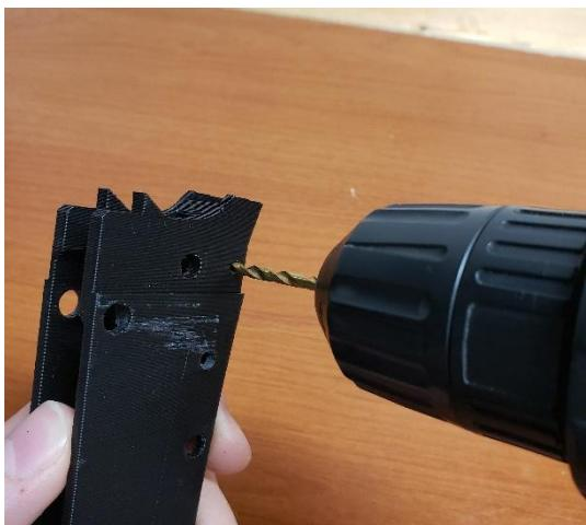
Next, use a 1/8" (3mm) bit for the trigger pin hole.
