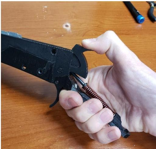
Hold the guide rod in place with your thumb, and use your other hand to pull the hammer back into the half-cock notch.
