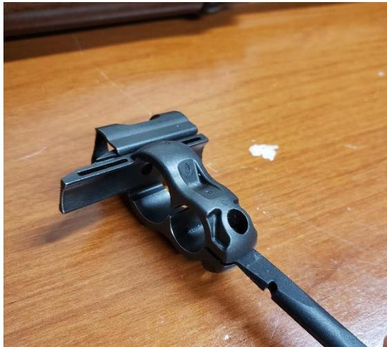
Next take your front sight and use a flathead screwdriver or similar to insert into the bottom and hold it apart for installation. The sight hood can also be slid off to get it out of the way.
