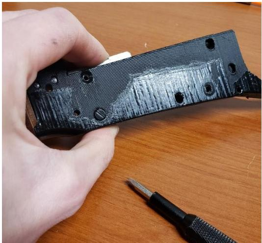
Hold the carrier in place and install screws.
