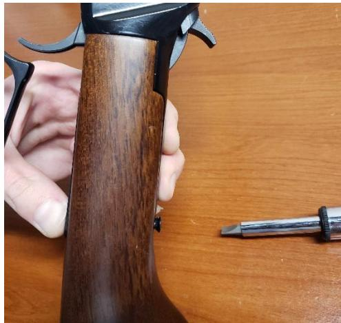
Hold the tang up and install the stock screw. Don't forget to install your inner mag tube as well.
