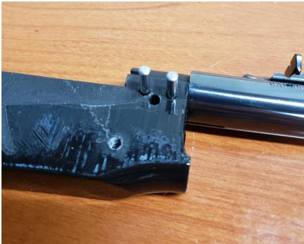
Next make sure your barrel is lined up and insert your two taper pins from the right side of the frame.
