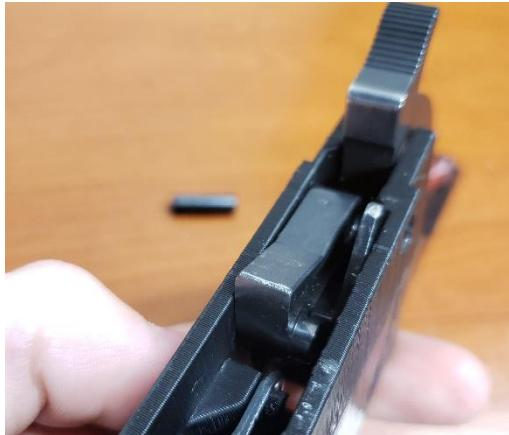
Put in the locking bar making sure the round lug goes underneath the lever. You will have to carefully press it down while you install the pin. Once the locking bar is in, check the function by opening and closing the lever. The locking bar should drop down when the lever is opened and pop up when closed.
