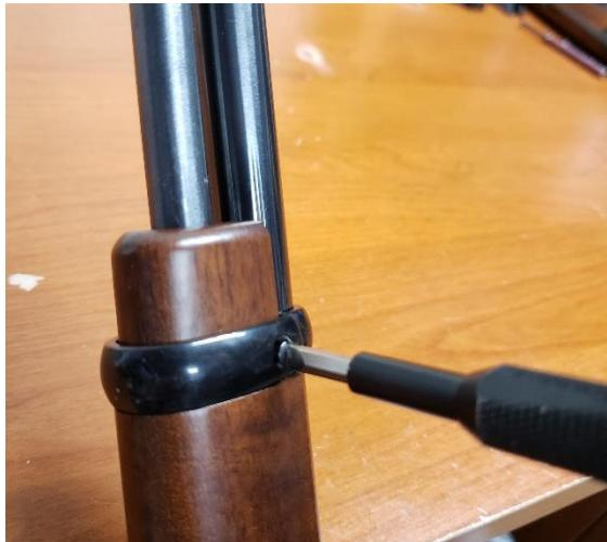
Insert the barrel band screw.
