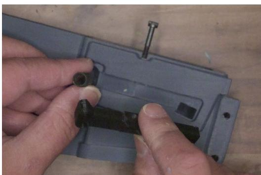
Insert the magazine release and magazine release spring.
