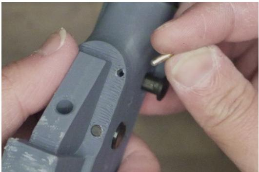
**Insert the rear takedown detent and spring into the channel, with the rear takedown partially inside the lower.**
