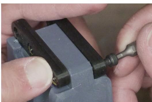
**Hold the left standoff as shown against the receiver, and screw in the bottom M4x20mm/30mm into the nut.**
