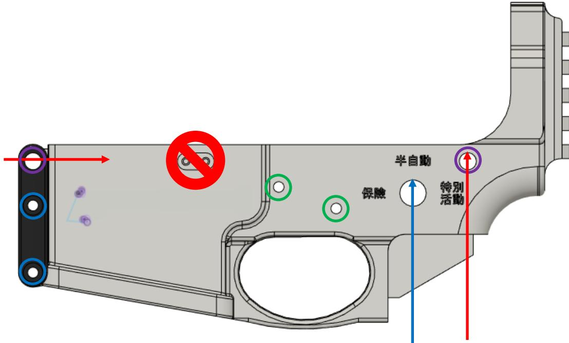
Use a drill bit to deburr and chase out the highlighted holes above.
