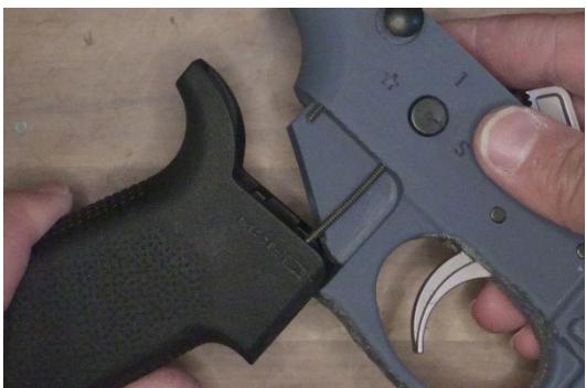
**Place the fire-control detent spring into the grip and prepare to put attach it to the lower as shown.**
