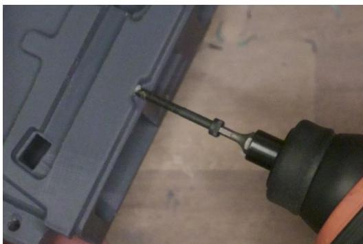
Insert the M3x30mm socket head screw and thread it partially into the magazine release geometry.
