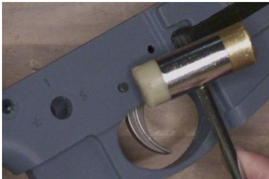
**Hold down the disconnector to align the hole with the trigger bow to the receiver, then drive a fire control pin through.**
