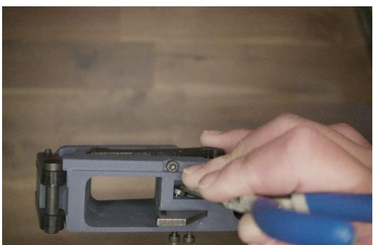
**Suspend the M3 nuts, and thread the screw further until it captures the M3 nut. Repeat this for the other screw.**
