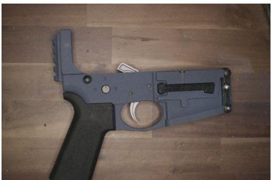
**Ensure that the rear takedown spring and the fire-selector detent spring does not kink as you attach the grip.**
