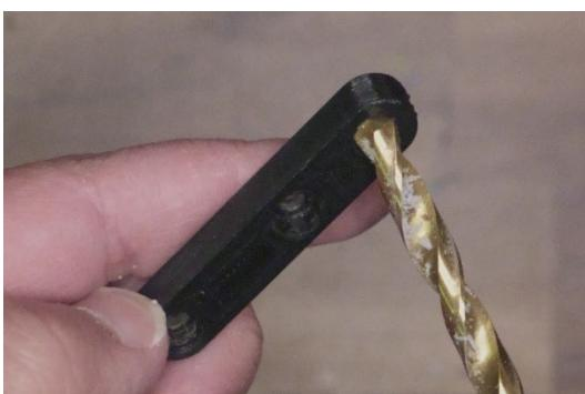
Using a 6.5mm drill bit, chase out the takedown standoff's takedown hole.
