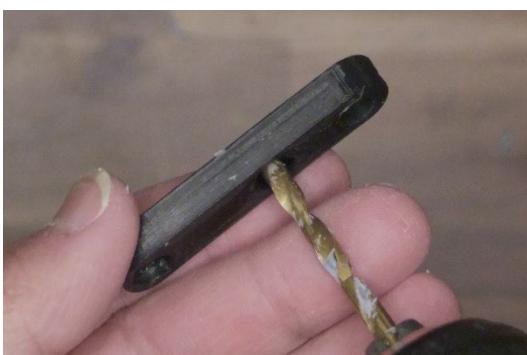
Using a 4.0mm drill bit, chase out the takedown standoff's M4 screw holes.
