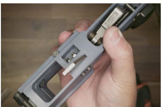
**Torque down the M3 socket heads, ensuring the M3 nut is tight against the receiver internally.**
