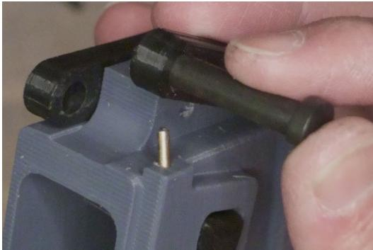
Insert the takedown spring and detent into the channel. Insert the takedown into the standoff, then pivot the standoff onto the detent.
