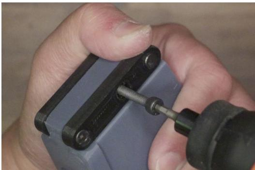
Screw in the remaining M4x20mm/30mm screw, while holding down *both* standoffs.
