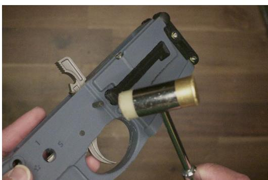
**Likewise, do the same for the hammer. Reset the hammer after you insert the pin completely.**
