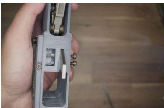
**Insert the ejector, lining up the holes with the screws, then thread through the ejector.**
