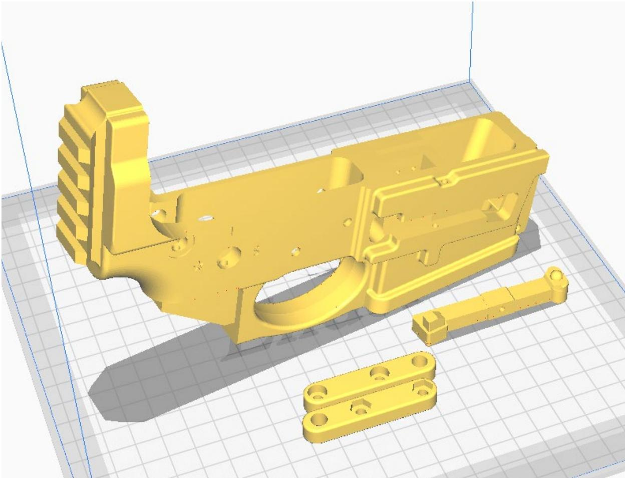
Print using the above orientation. Use Cura's "Align Face to Build Plate" tool under "Rotate" to orient the lower receiver with the magwell facing downwards onto the build plate.
