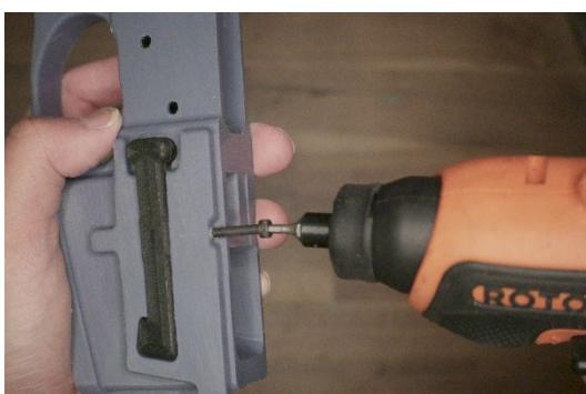
Thread the M3x30mm socket head completely, until the socket head is flush with the top of the receiver.
