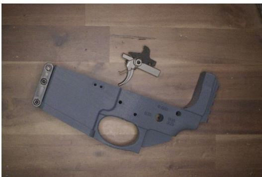
Prepare the AR-15 trigger. Insert this into the fire control pocket.
